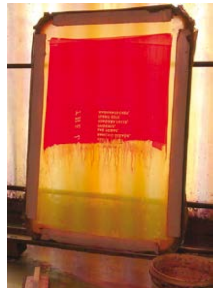
Emulsion removed from half of the screen
