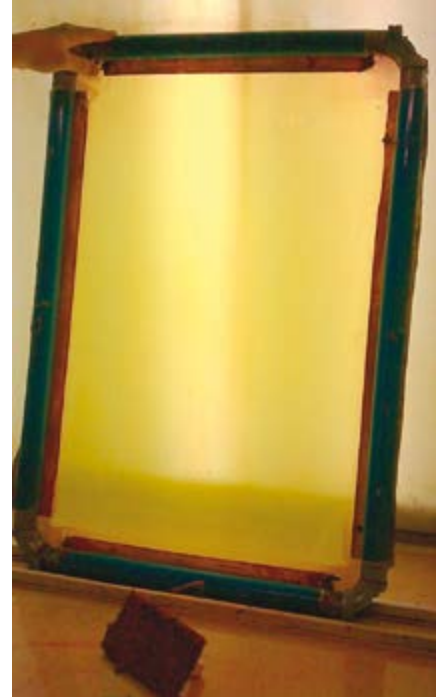
A clean screen with no staining present
