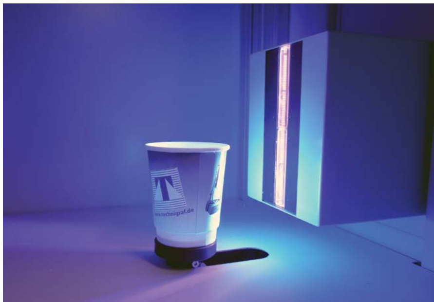
Rotative curing with Technigraf's Aktiprint B compact LED UV dryer. Single-side material feeding and output enables fast curing of UV inks or coatings on containers or moulded parts made of plastic, metal or glass
