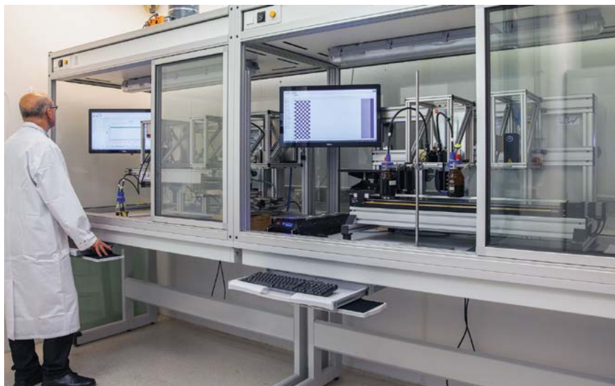
Figure 4: A modular 3D inkjet printing unit from VDW-Consulting. The printer is compatible with a range of industrial printheads such as Xaar, Toshiba-tec, Fuji Dimatix, Ricoh, Konica Minolta and Kyocera
