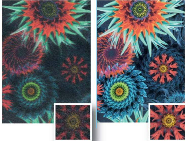
Digital pigment printing on polyester fabric without primer (left) and with CHT's Tubijet primer (right)
