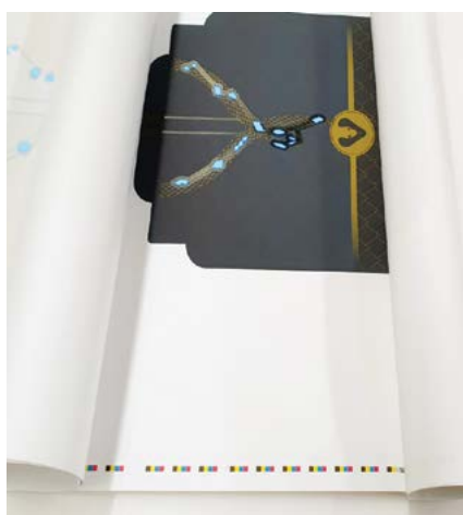
Figure 2: Saralon's latest development in the field of Electroluminescent technology: printed 'light' on paper
