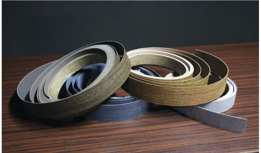
UV inkjet printing is a cost-efficient alternative to gravure printing for edge band production
