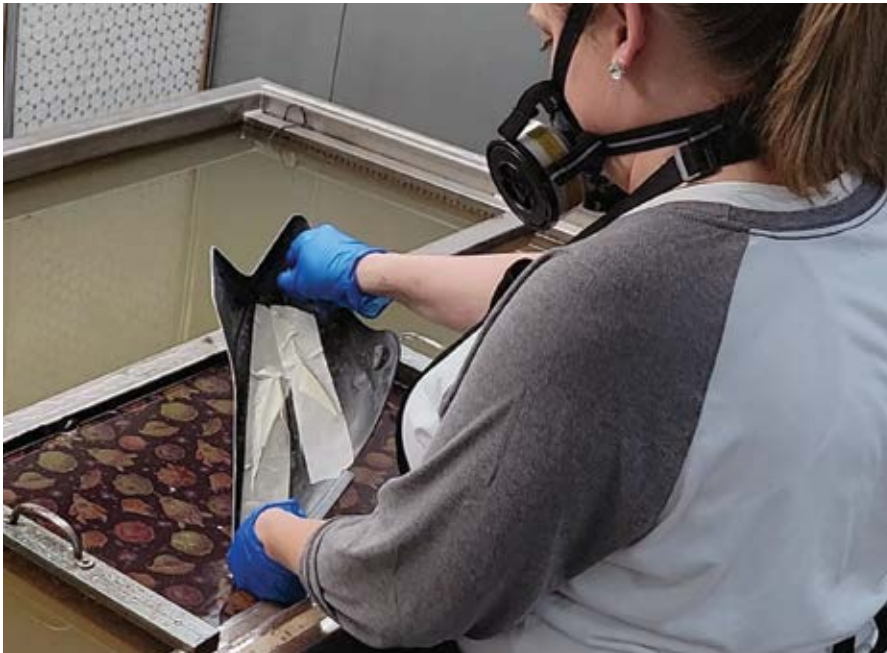
Hydrokon on water's surface prepared for dipping
