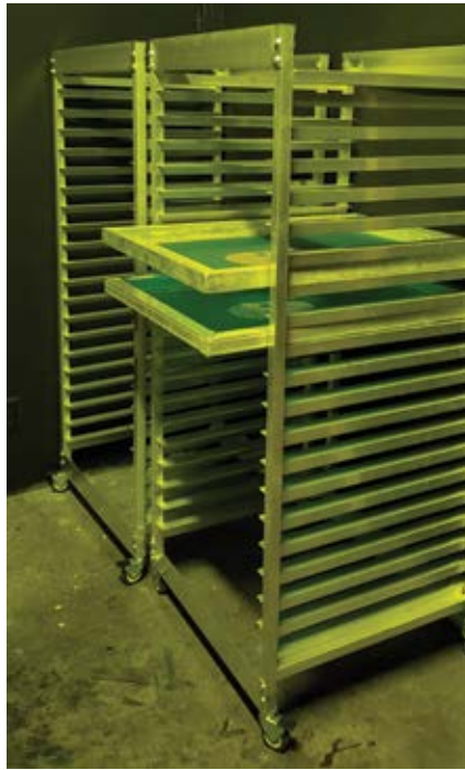
Coated screens stored shirt side down to get the best emulsion coverage
