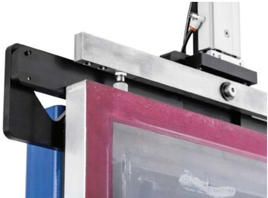
Above and below: Pin-registration system on the computer-to-screen MHM SPYDER II
