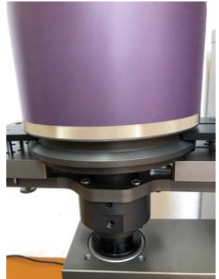
Welded to a round shape, the Mega Screen is then attached into the stencil ring (source: Gallus Ferd. Ruesch AG)
