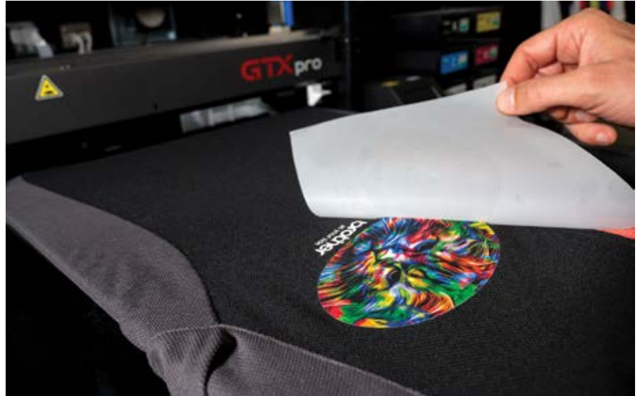
Foil removal after pressing the printed sheet onto the garment
