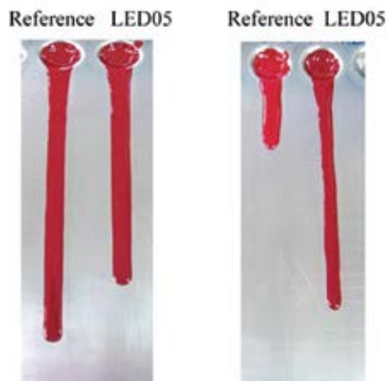
Figure 8: Flow of flexo ink with reference amino acrylate or LED 05 (left: one day storage at RT; right: four week storage at RT)
