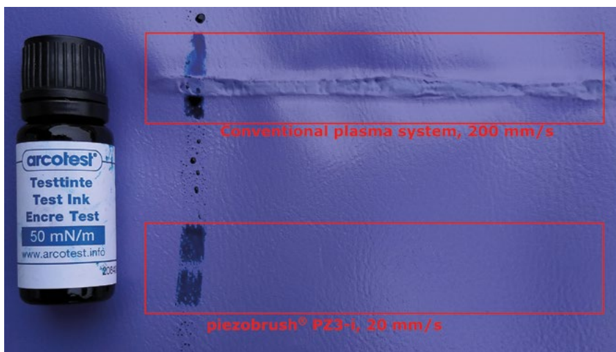
Figure 3: Comparison of plasmabrush PB3 and piezobrush PZ3-i on a temperature-sensitive film
