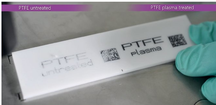
Figure 2: Adhesion test showing results of inkjet printing on untreated and plasma-treated PTFE with the piezobrush PZ3
