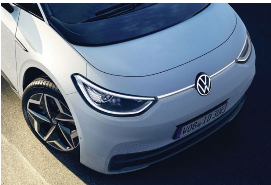
Radome device reflects the brand and is also transparent to radar and or lidar technologies
