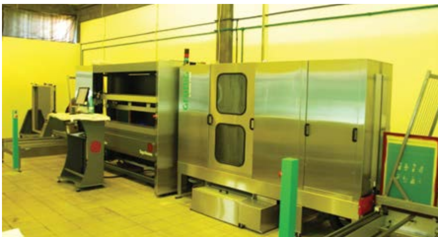
Digital direct light stencil exposing in-line CtS system – 1270dpi
