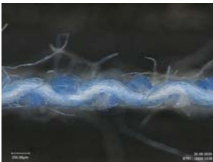
Fig. 3a: Cross-sectional image of a digitally-treated textile using minimum dot size (treatment made visible by blue colour)
