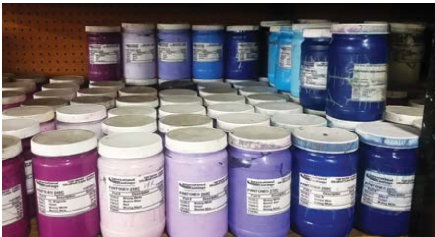
Pantone Colour ink matches, labelled with formulas printed from International Coatings' online PMS formulation site
