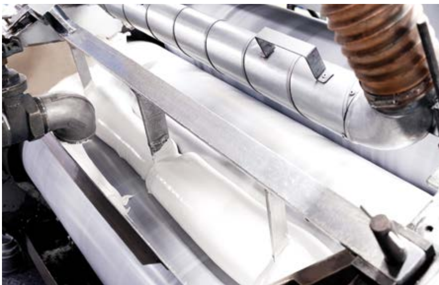
Triple roll mill white ink. Using the latest analytical equipment ensures ink formulations can be precisely controlled
