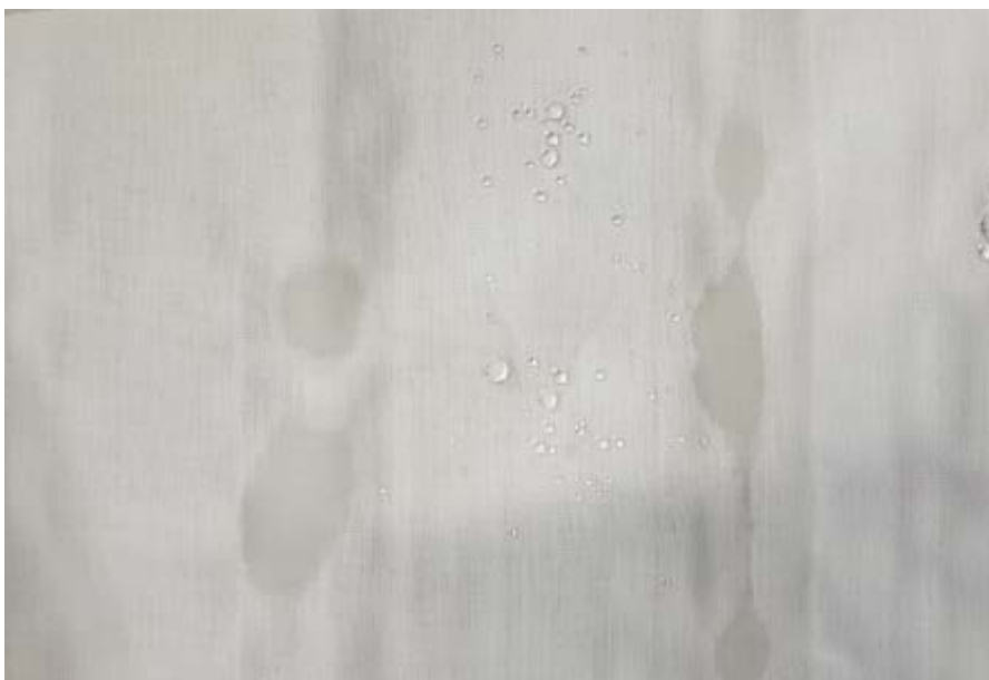
This textile has been digitally treated with chemistry formulations to obtain both hydrophobic and hydrophilic properties. Water forms droplets with high contact angle on hydrophobic areas, whereas on hydrophilic areas the water penetrates the material
