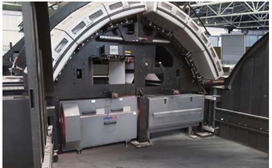
adphos' upgrade kit for HP's T400 inkjet press can increase printing speeds by up to 60%, according to Inkjet Insight's study
