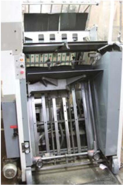
A die-cutting machine presses the printed sheet and the die together to cut out shapes
