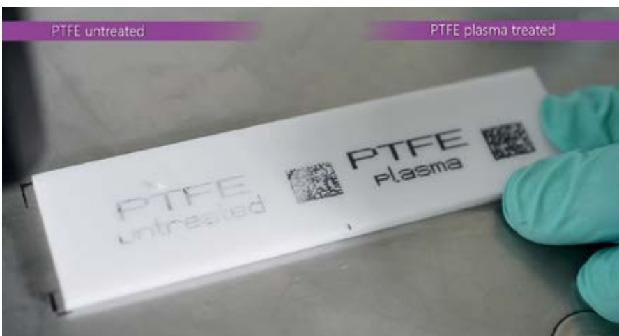
Adhesion test showing results of inkjet printing on untreated and plasma-treated PTFE with the piezobrush PZ3
