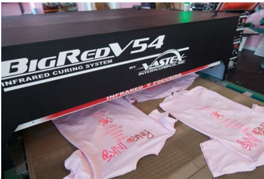
The 137cm wide belt and large heating chamber of the dryer can handle more than twice the number of shirts than the previous 76cm wide dryer
