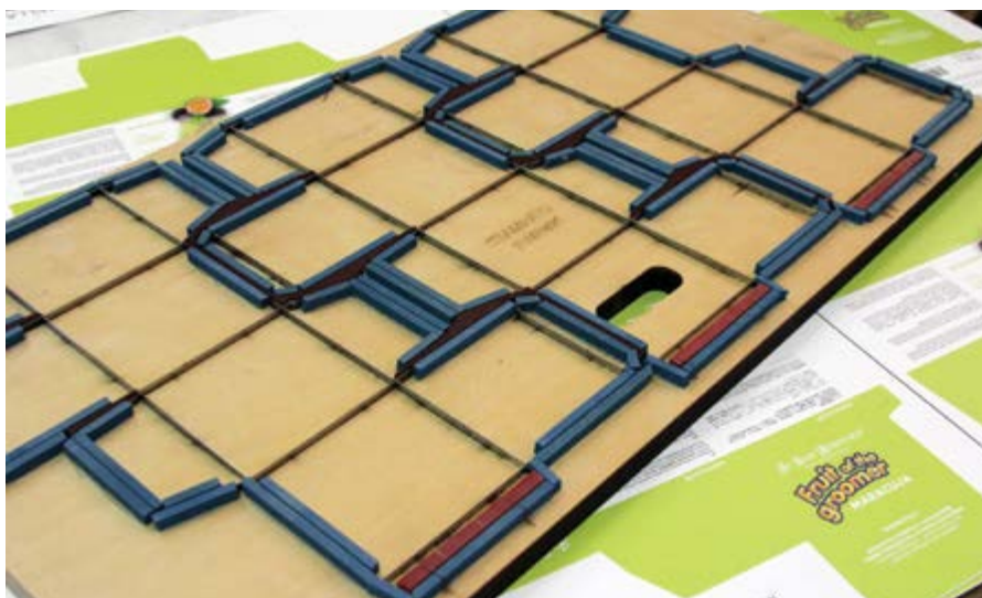
Die cutting is a quick and inexpensive way to cut and score large quantities of identical printed items
