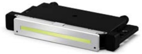
The new small form S800 printhead from Epson is equipped with 600 nozzles per inch, with a 1mm distance between nozzle rows
