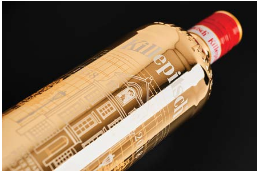
Screen printing offers options from printing on simple round bottles with thermoplastic inks to 9-colour printing on difficult shapes with UV or LED curing inks
