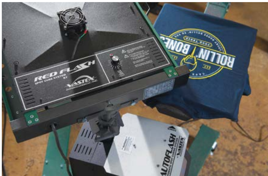
A foot pedal rotates the flash cure unit into place above the newly printed colour, and then automatically rotates away, preventing over- or under-flashing
