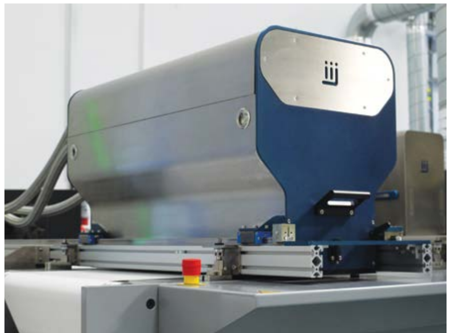
Industrial Inkjet's Colour Print 562 print engine is one of the company's largest print widths, used mainly in wide web or sheet fed applications such as security printing, décor print or packaging
