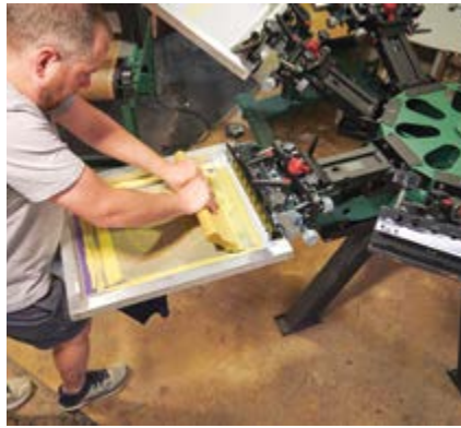
Advance Stamp & Sign prints shirts and hoodies for local businesses and schools, and clamps a 51 x 66cm vacuum pallet onto the press's pallet arm to print signs up to 46 x 61cm
