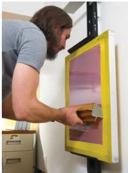
C100 screen coater rack frees the operator's hands to coat the screen quickly, easily and uniformly
