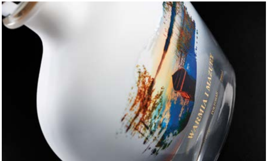
A result achieved with dual process: hot stamping + screen printing
