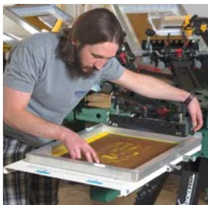
VRS pin registration system allows screens to be registered off-press, and then clamped on press with all colours in register
