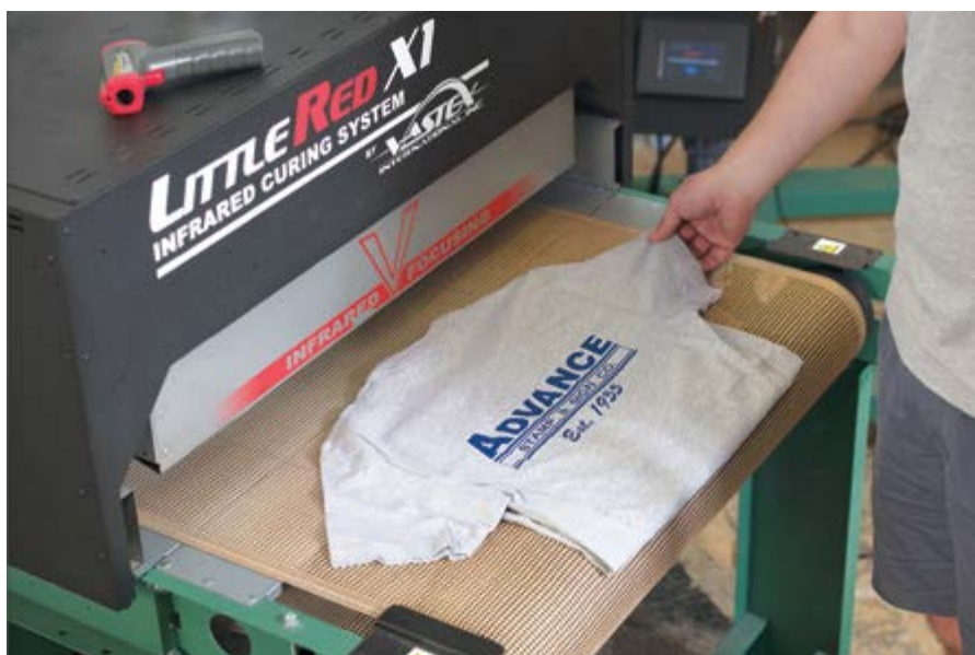
The 76cm wide infrared conveyor dryer can cure up to 130 plastisol-printed images per hour
