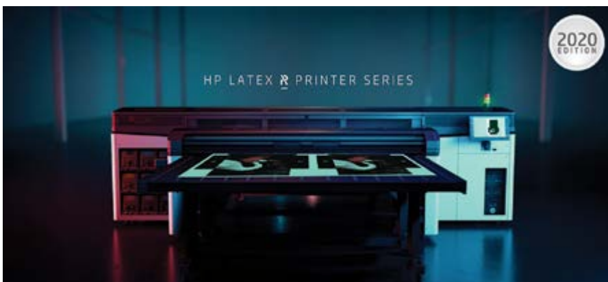
A hybrid printer with both roll and rigid capabilities, HP’s Latex R Series features white ink that is compatible with wood and acrylic
