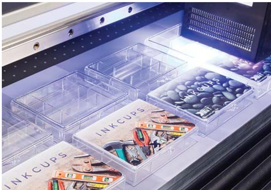
Bi-directional printing of plastic boxes utilising a specialised ink
