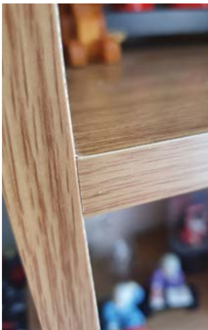
Example of an edge band – the strip of colour-matched tape often found on the edge of furniture
