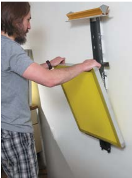
C100 screen coater rack frees the operator's hands to coat the screen quickly, easily and uniformly
