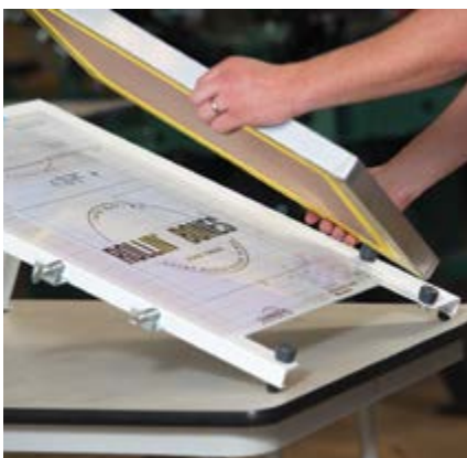
VRS pin registration system allows screens to be registered off-press, and then clamped on press with all colours in register
