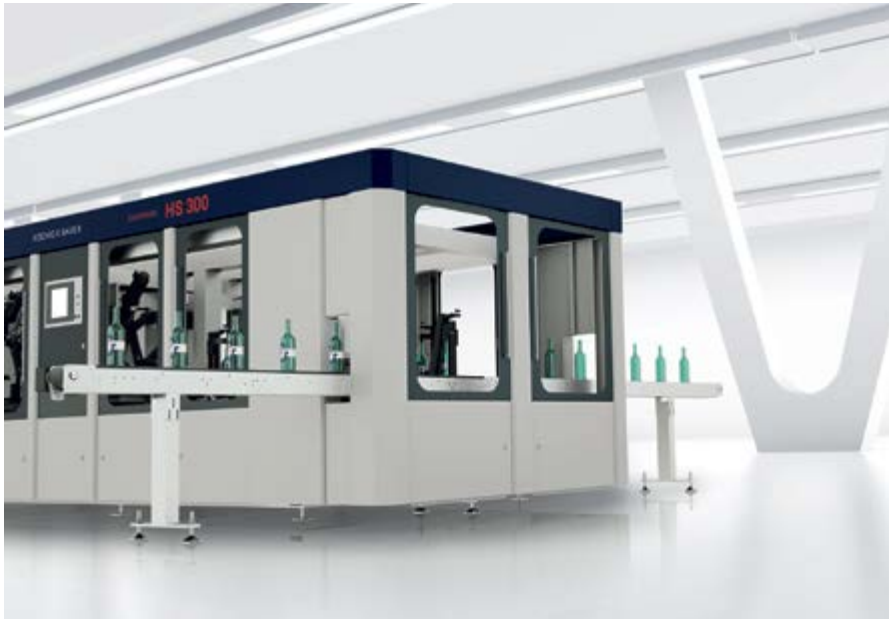
The HS 300 is Kammann's new high-speed printing machine for the decoration of round beer bottles and glass bottles for soft drinks
