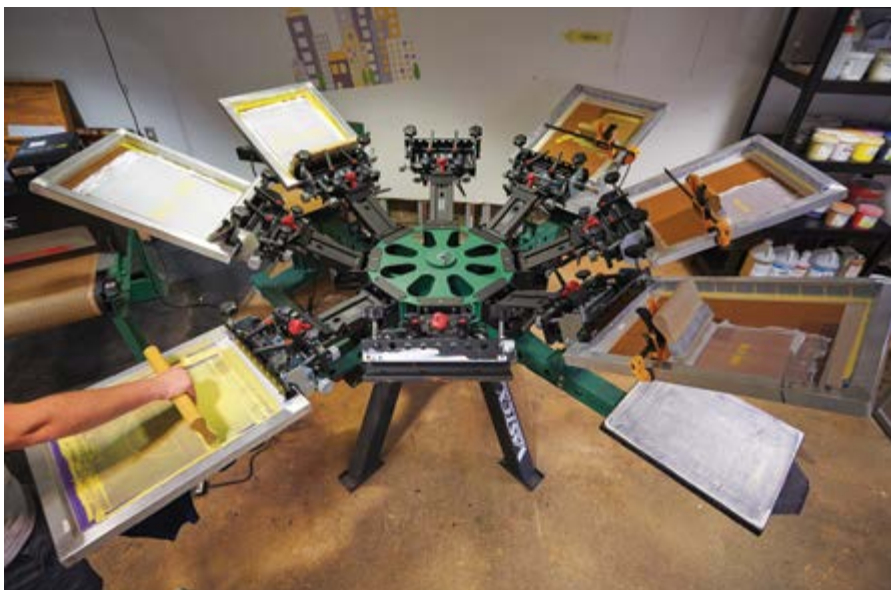
Advance Stamp & Sign upgraded its 4-colour/4-station manual press to 8-colours/8-stations in a few hours
