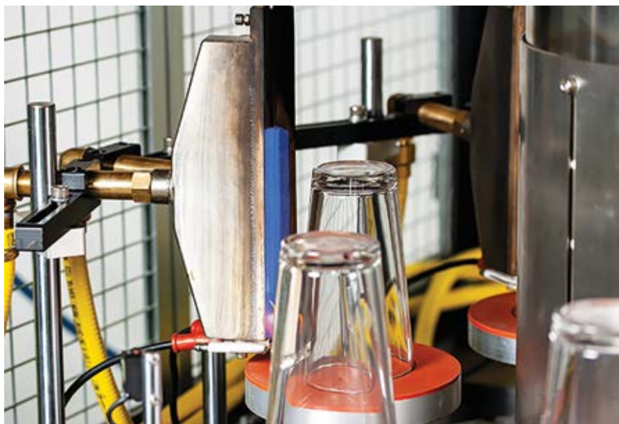
To obtain optimal adhesion, glass needs to be flame-treated. In this case, the glass comes into contact with the hottest part of the flame to adjust surface tension
