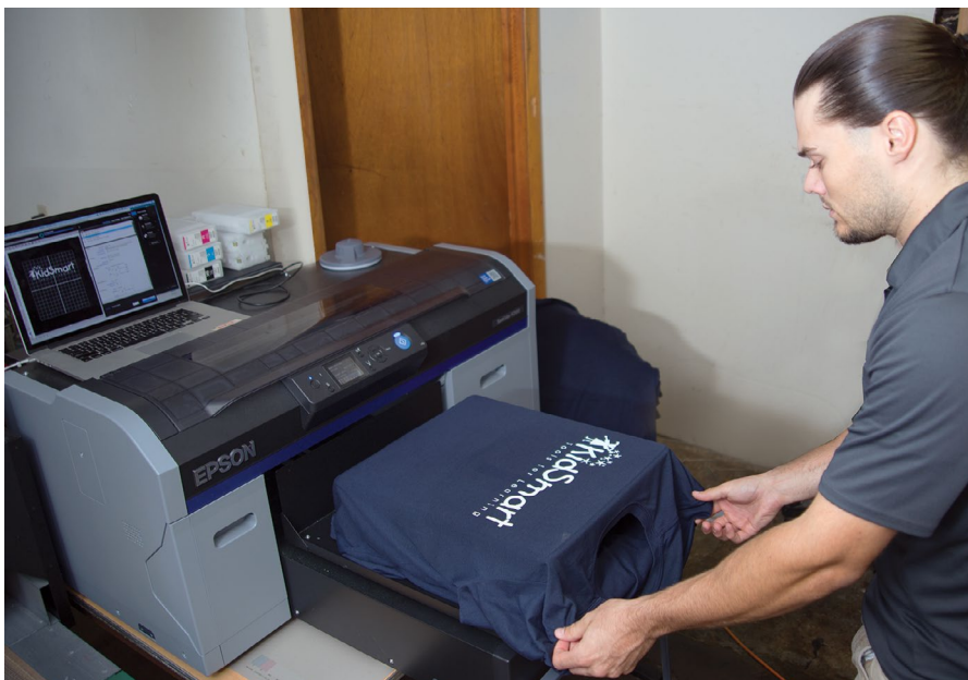
DTG-printed shirts looked great coming off the inkjet printer but former heat pressing muddled the colours
