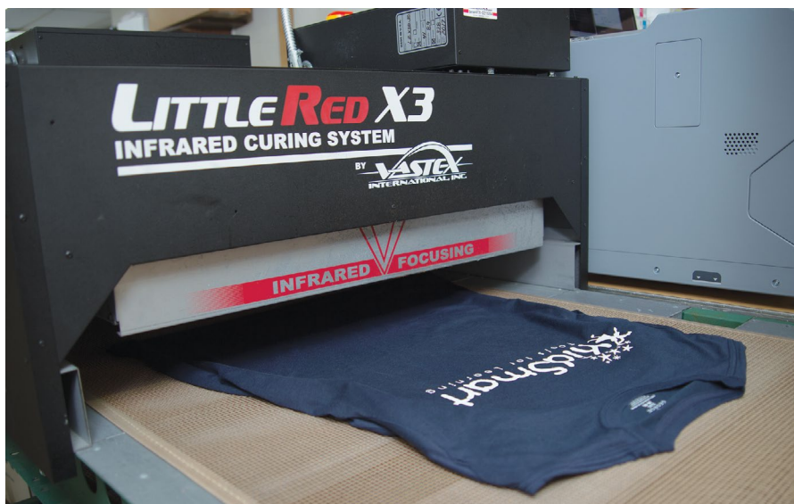
Three 61cm-wide infrared heaters are height adjustable, allowing images to be positioned at an optimum distance from the heaters regardless of garment thickness
