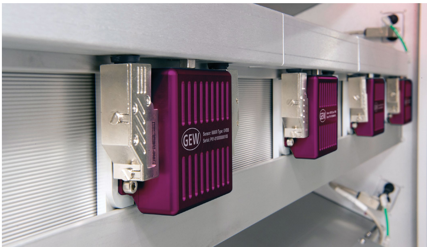
Multi-point monitors continuously measure UV intensity across the web, making it possible to generate a UV curing certificate for every batch
