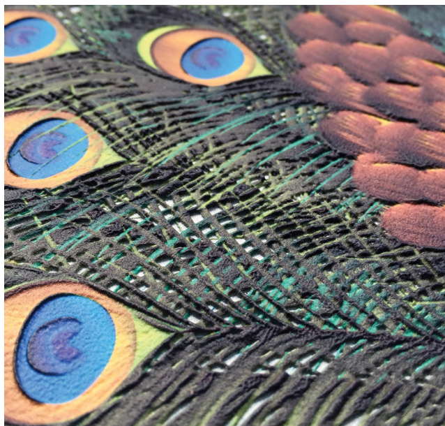
Layers of ink being used by an LED UV printer to create textured finish
