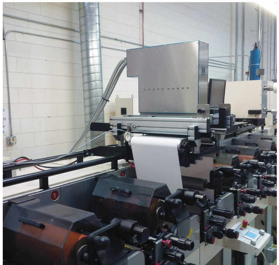
IJJ print engine on a flexo base
