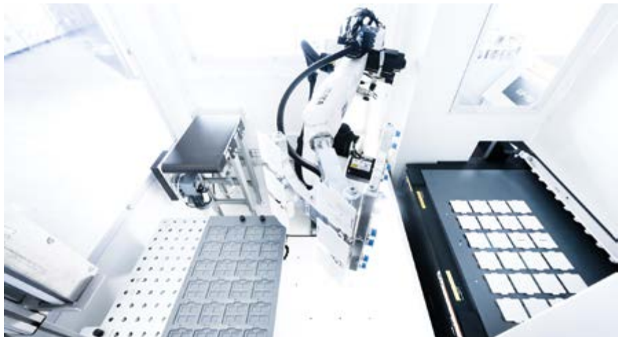
Inside the robotic cell; a Kuka Cybertech nano KR 10 robot equips a Mimaki UJF-7151 Plus UV inkjet printer with objects to be printed
