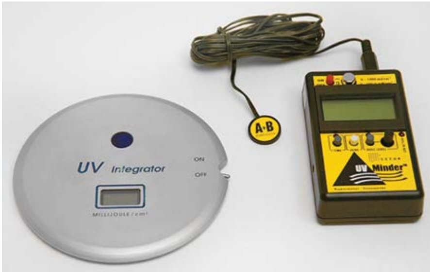
With a radiometer the effectiveness of the exposure bulb can be checked
