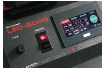
The LED-5000's digital control system simplifies exposure settings
