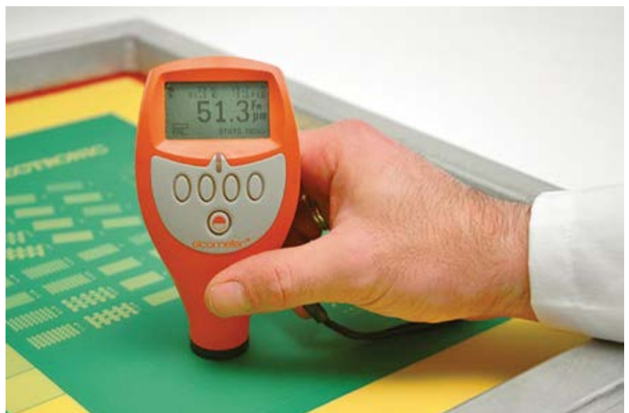
Measuring thickness with a thickness coating gauge
