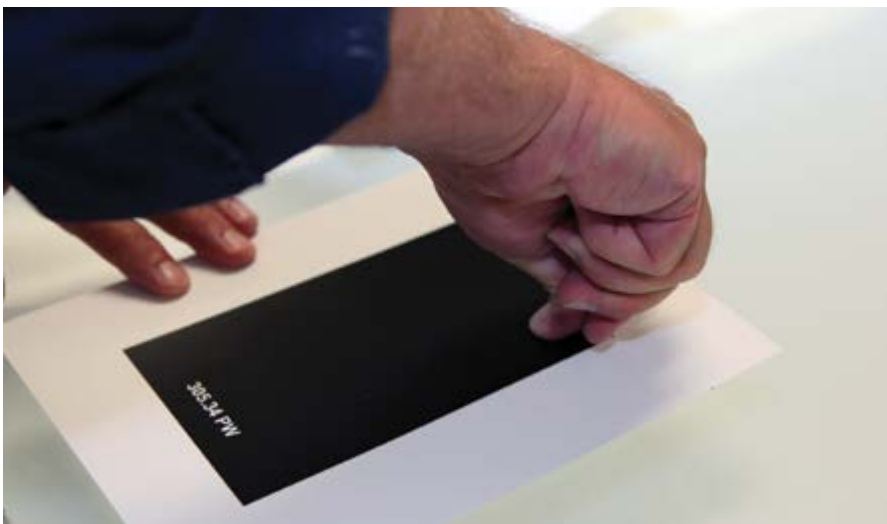
No matter the chemistry of the ink used (solvent, UV, etc.), a thumb twist test should be performed after printing to check for adequate dryness or initial cure of the ink
