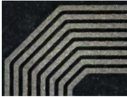
The printed lines which form part of an electric circuit. They are greatly magnified and show just how precise the printing needs to be
