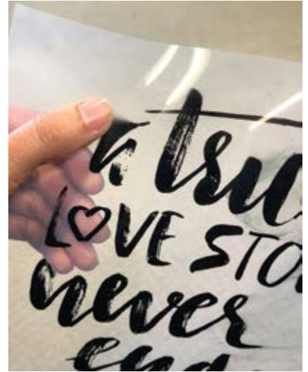
Temperature and humidity will affect how the ink dries on the ink jet film
