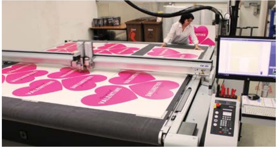
Tandem operation lets the Zünd G3 3XL-3200 cutter produce non-stop
