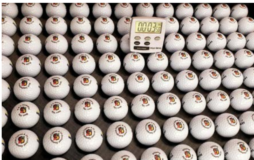
It takes three minutes to print this tray of golf balls using a UV-LED printer
