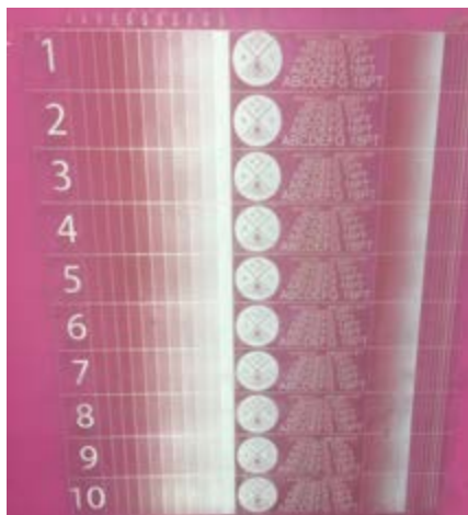
Fig. 5: Exposure test wash out, ready for examination
