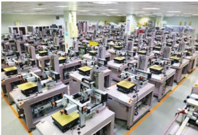
Mass production at the ATMA factory in Taipei, where camera controlled systems print glass covers for mobile phones
