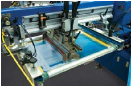
Screen printing applications require increasingly higher quality squeegee blades to meet their demands
