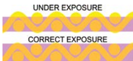
An underexposed screen will lose crucial emulsion on the squeegee side
