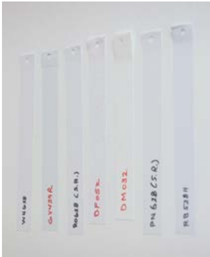
Test three to five clearly identified/labelled 1x10-inch sample strips of material
