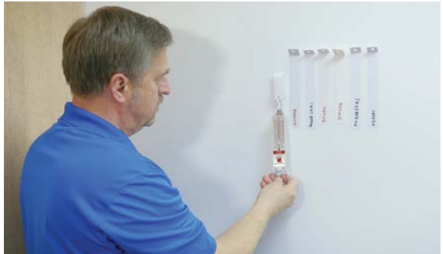
After 30 minutes, use a spring scale to measure adhesion
