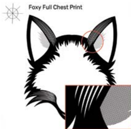
The Foxy Full Chest design was film printed with a very clean lower line screen. Zoomed in to show the open space around each spot making printing dot gain friendly
