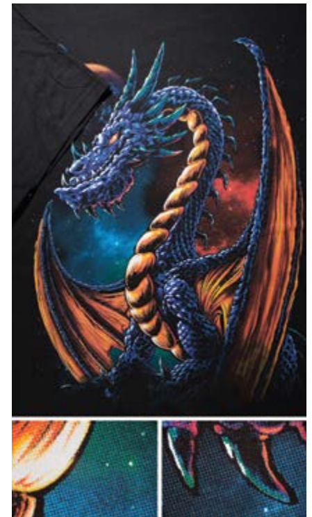
This image shows inks printed wet-on-wet, dot over dot (single angle flamenco style)
