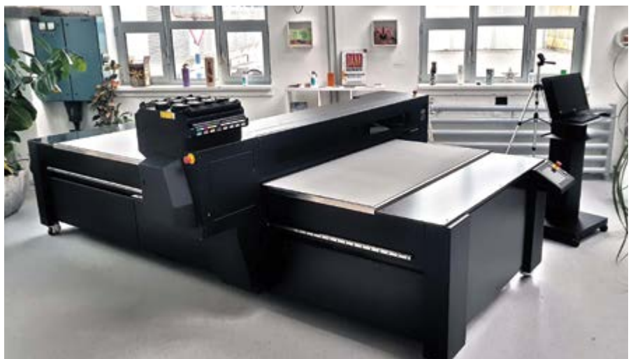
The new Matrix R platform from Azonprinter is based on Ricoh Gen5 printheads
