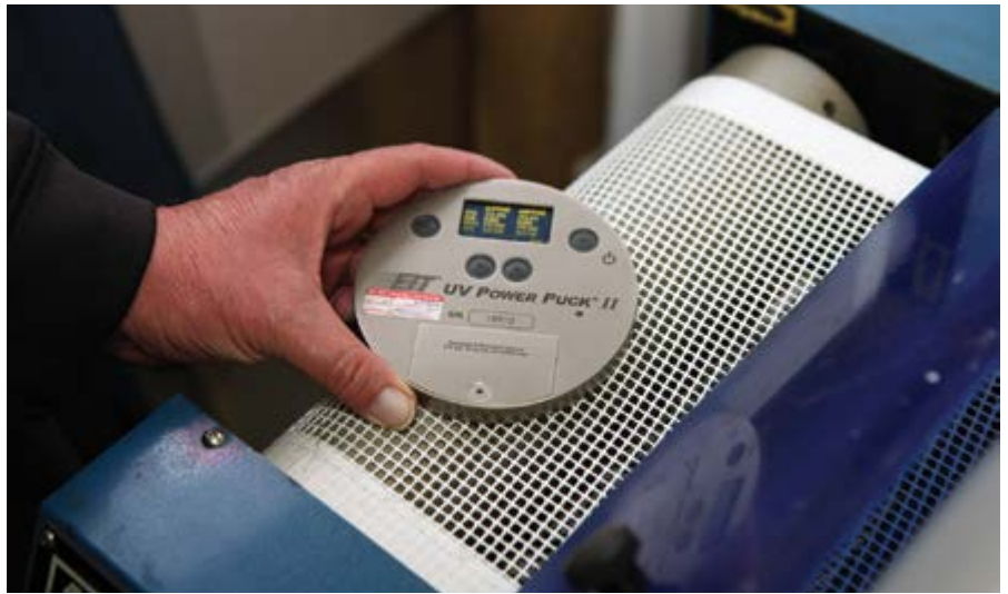
Confirm cure unit energy output with a regularly calibrated radiometer
