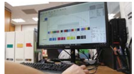
PressTune shows a summary of the quality score of the various parameters of a job, as well as the overall job score. It also provides insights on each measured press sheet for the various quality parameters such as lab value, density, tonal value increase, production mode, measurement, and score trends
