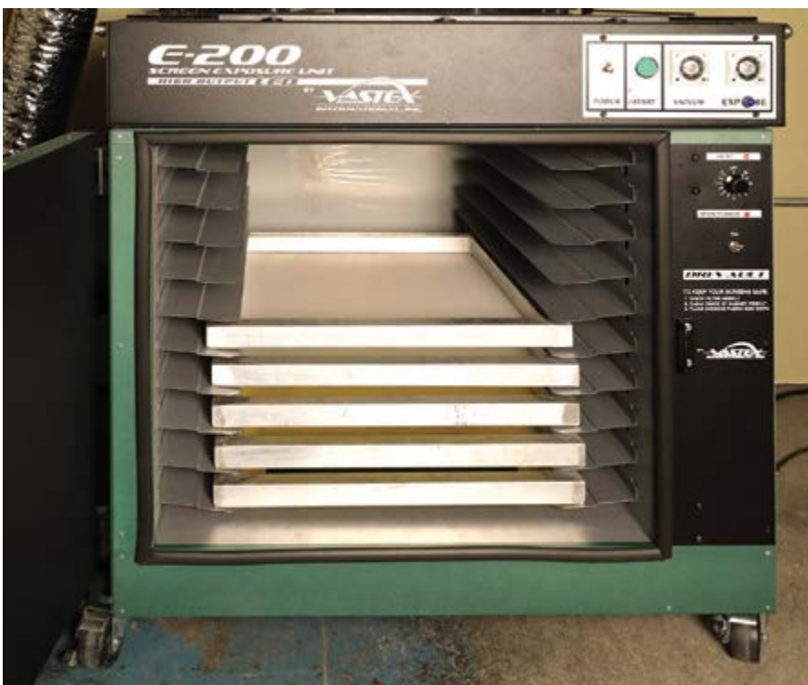
An enclosed drying cabinet with controlled, heated and filtered air flow and horizontal drying racks offers the best way to finish drying screens
