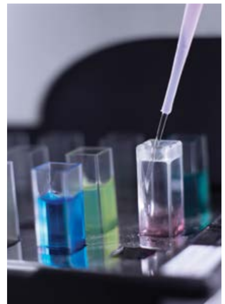
Ink samples prepared for particle size analysis, a critical specification for printhead performance
