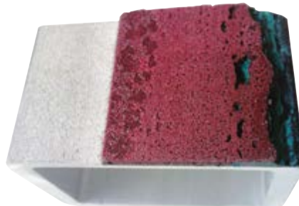
Figure 2: Cleansed aluminium frame profiles before and after treatment
