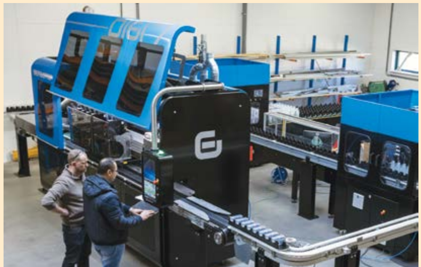
DIGI 7 Single Pass automation with loading and unloading system
