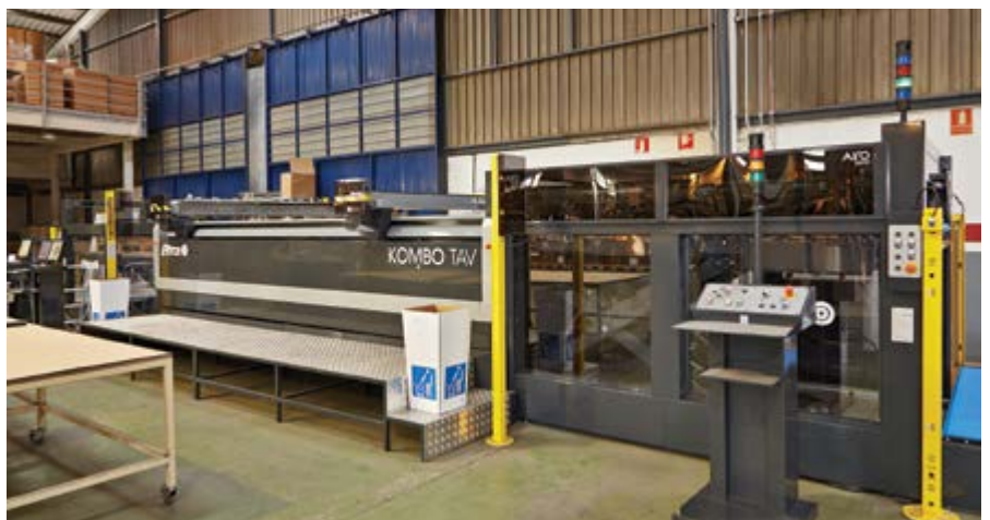
Elitron's fully automated digital cutting solution Kombo TAV-R with the special web-to-print configuration
