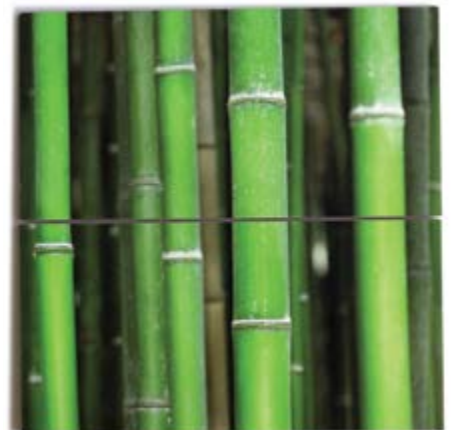
This printed glass was pre-treated using the pyrosil process and a silane-based primer to guarantee adhesion also under humid conditions. The UV ink printed on top provides excellent chemical and mechanical stability. (Image courtesy of Tiger Coatings)
