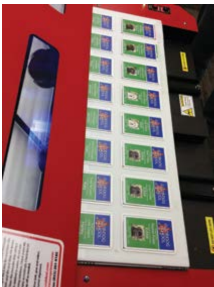
Printer producing finished ID cards with variable data and photos
