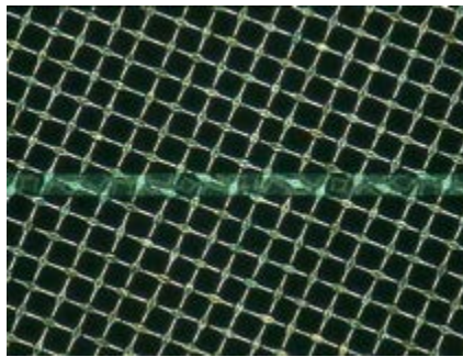
Figure 10b: 50-micron negative line on 360 .0006 wire mesh
