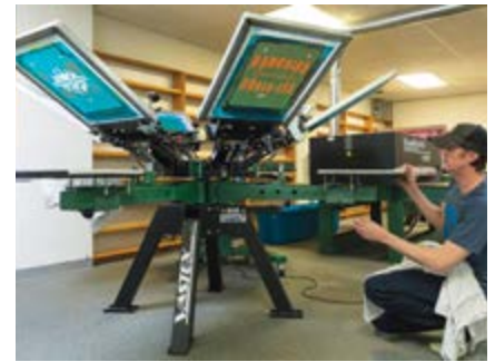
Micro-registration allows fine-tuning of registration and off-contact of the V-2000 print head
