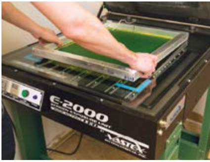
The E-2000 LED screen exposure unit with vacuum hold-down exposes screens in 10-20 seconds
