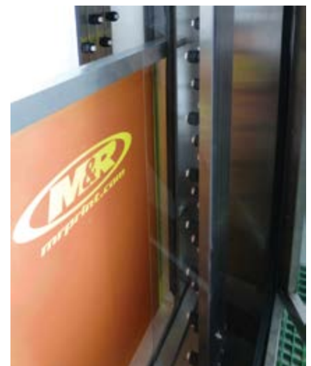
Balanced pressure and even application provided by nozzles on both sides of the screen clean consistently and help maintain screen tension and extend screen life
