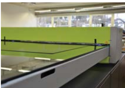
The XPS Crystal delivers both back and main exposures onto a flexo plate almost simultaneously
