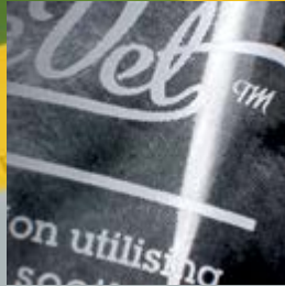
Outstanding printing quality of fine halftones on tubes printed with SEFAR® PCF FC 180/460-27Y
