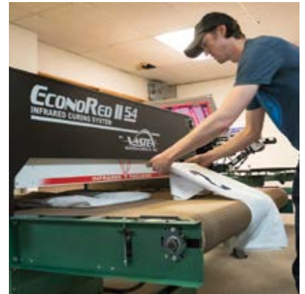
Art-Fx signs & Graphics feeds the output of two presses to an EconoRed II 137cm wide infrared conveyor dryer
