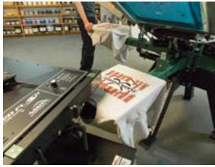
The Auto-Flash function of the Red Flash unit rotates the heater away from the pallet to prevent over-flashing.
