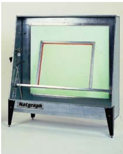
Dedicated washout booth with white light backlight (Image courtesy of Natgraph Ltd)
