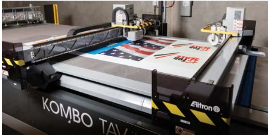
Kombo TAV-R uses twin gantries controlled by TwinCut software
