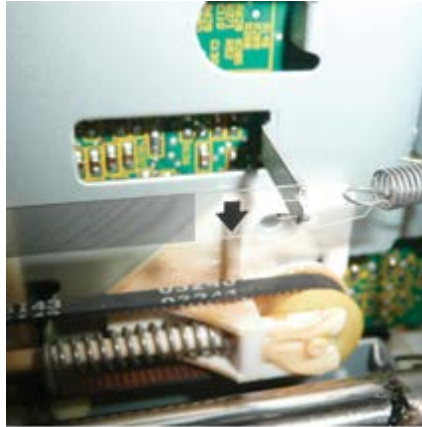
A linear encoder (left) and a rotary encoder
