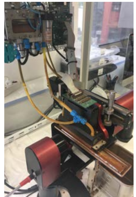
Drop watcher with a stroboscope (resolution 1292x964 pixels) calibrated at 1 micron catches drops in flight
