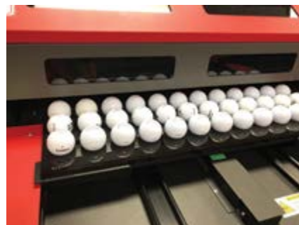
Allow for the size of a jig or support mechanism if printing golf balls
