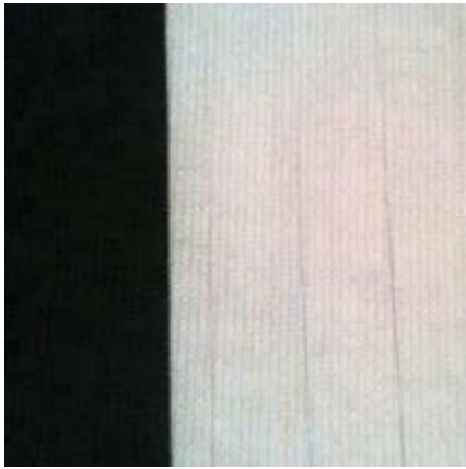
An example of printed vertical lines caused by a dirty encoder strip
