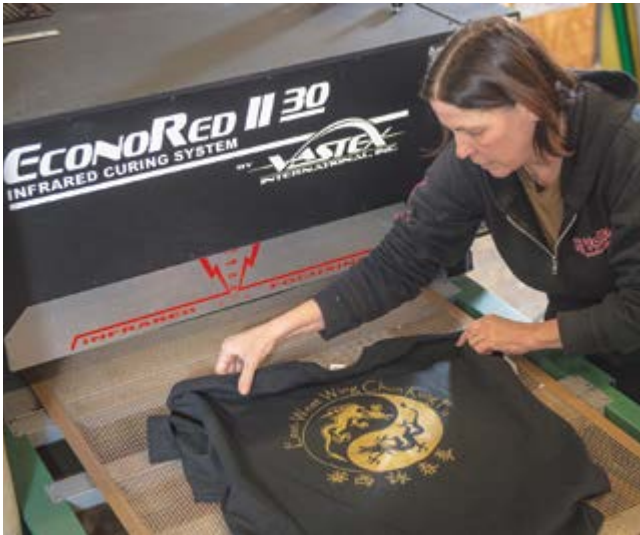
Loading garments onto the 76cm wide belt of the EconoRed II 30 infrared dryer
