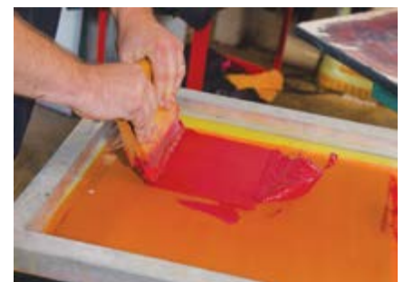
Prints a single-colour image onto a sleeve tacked onto a V2-Series sleeve pallet
