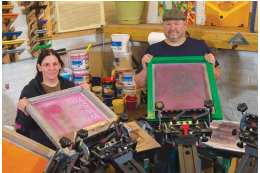
After the eight-colour/eight-station upgrade to the V2000HD press multiple jobs can be run simultaneously with different size pallets
