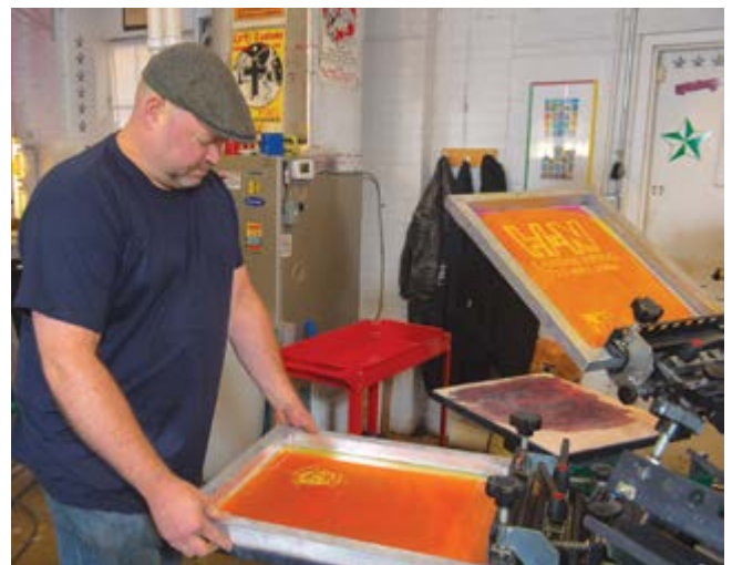
Locking the print-head into a registration gate ready for printing
