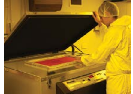
A self contained screen exposure unit
