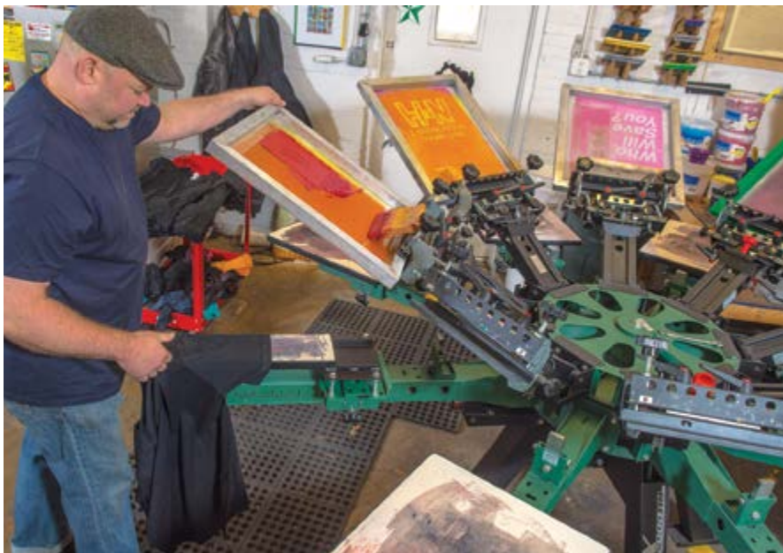
Mike Ritchey fits a shirt onto a sleeve pallet of his V2000HD eight-colour/eight-station press
