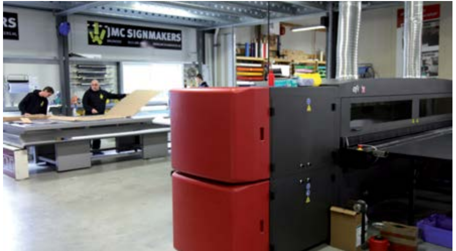
The EFI VUTEk GS2000LX Pro 2m production-level LED printer
