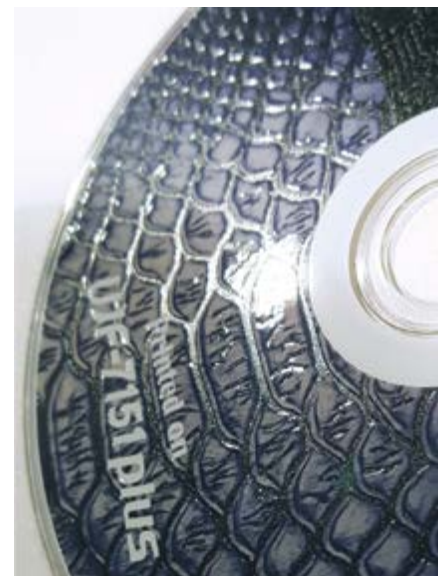
Texture on an object is produced using layers, in this case clear UV ink
