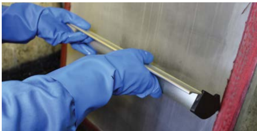
Use an old coating trough to apply the low caustic cleaners
