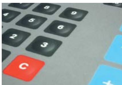
A typical screen-printed membrane switch panel
