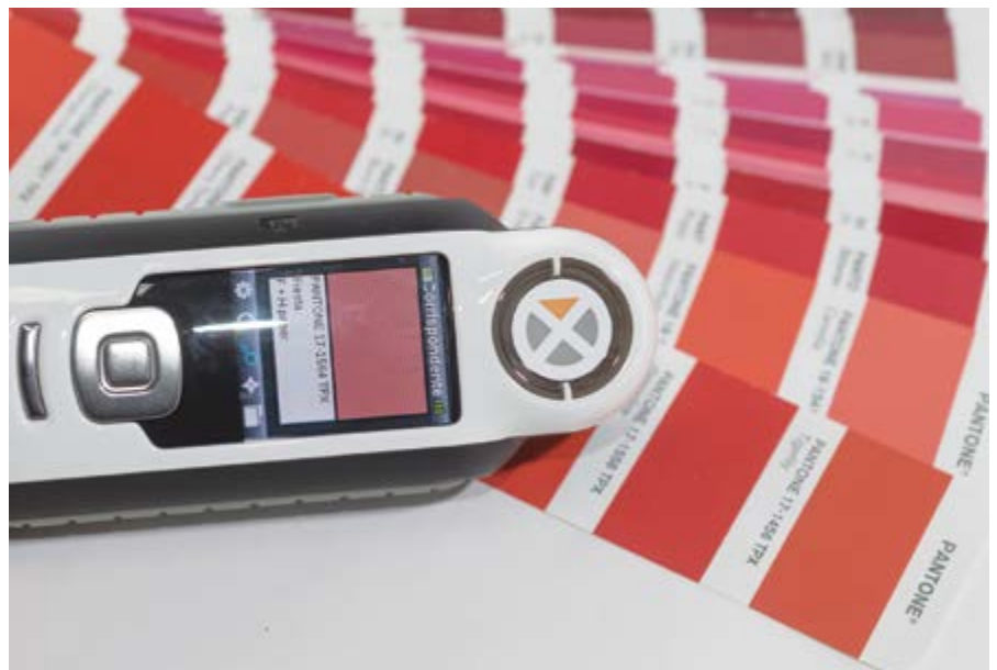
X-Rite's Capsure is a convenient hand-held instrument that captures spectral values
