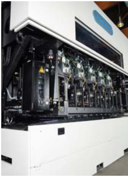
Figure 5: The core of Hymmen's digital printing know-how is in the ink units
