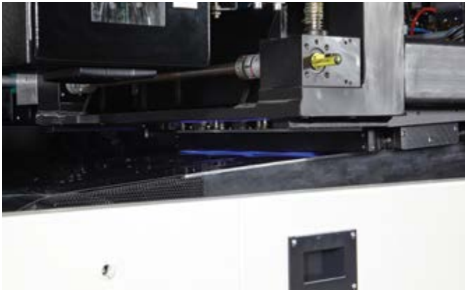
Figure 4: detail of the integrated UV drying of the surface and print-heads from the bottom
