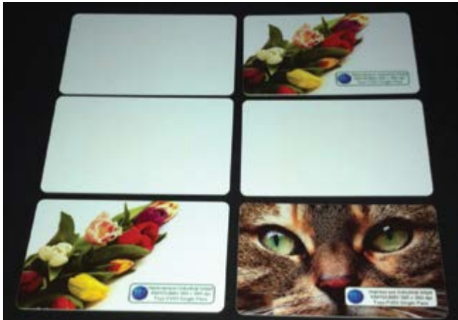
UV fluorescent security ink showing white light and with UV light – colour rebalanced
