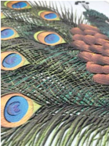
An example of textured printing. Textured 3D printing achieved by incremental raising of the print-head on each pass
