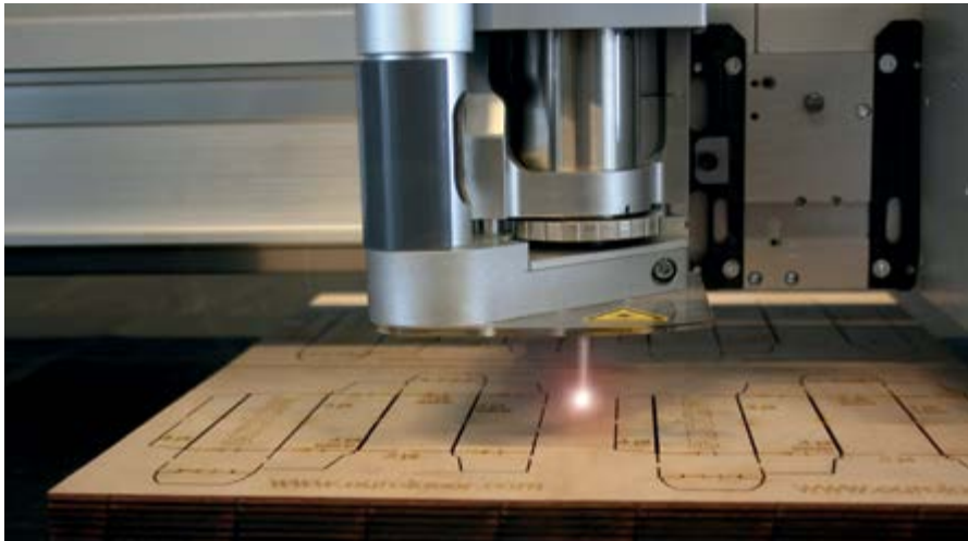
The work pieces are processed without contact and pressure using the bundled laser beam
