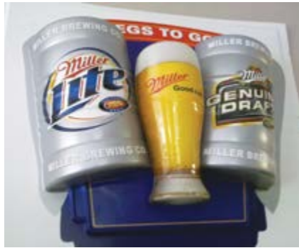
Deep draw thermoforming can be accomplished without cracking or mosaic features
