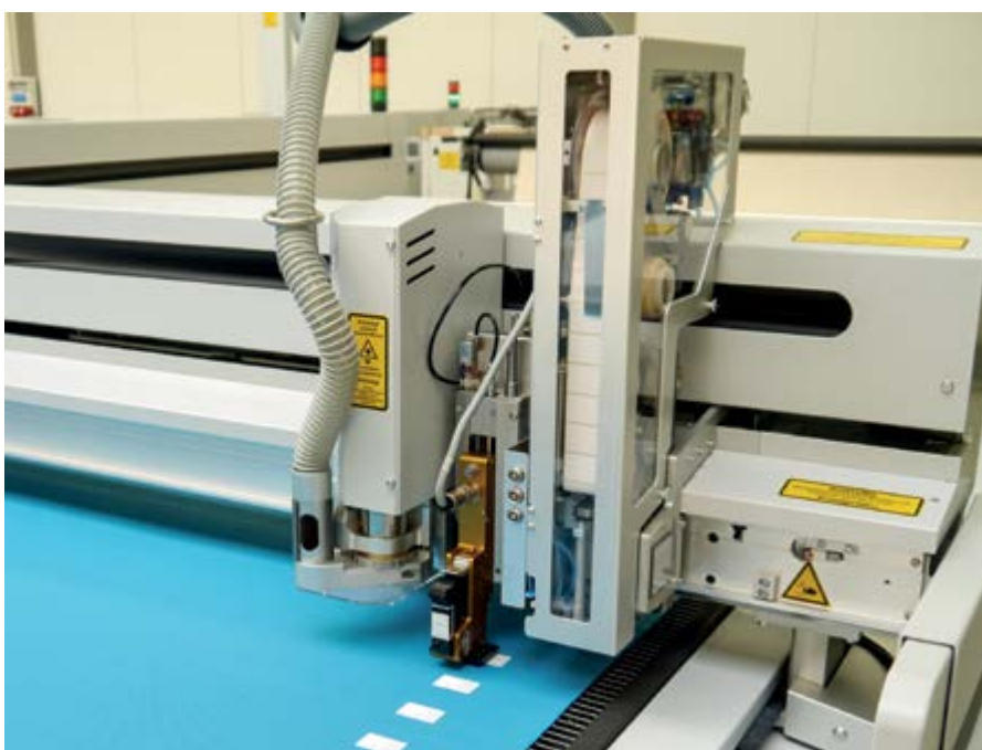
With the new label and ink printer module, users can place individual labels onto cut pieces for subsequent printing
