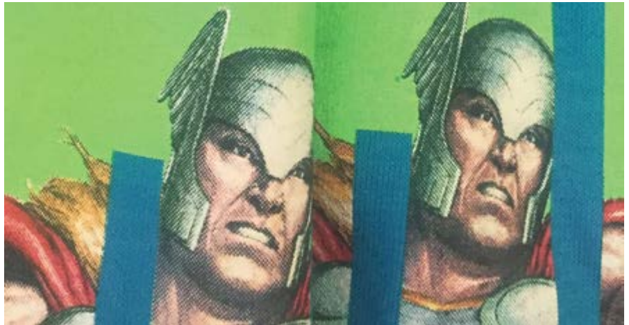
Figure 6 – better print results with thin thread mesh Picture courtesy of Allan Heller, Screen Creations, Mexico
