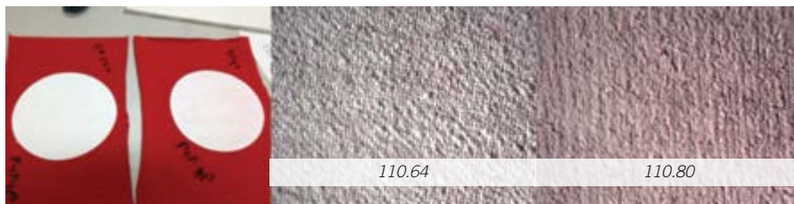
Figure 4 – comparison of dye migration of prints made with thin thread versus standard mesh (Picture courtesy of Eric Klein, Saati Americas Corp)
