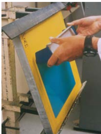
Learning how to coat a screen correctly with direct emulsion can take time
