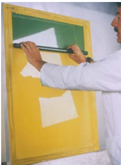
All three methods of applying capillary film require degreased screens
