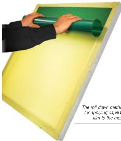
The capillary film contacts the screen, ending with the corner of the film being held
