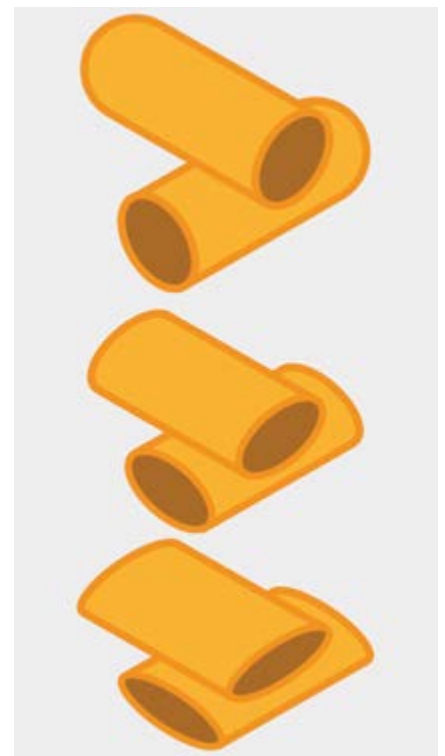
Figure 7: the 'same' diameter mesh becomes more elliptical going from stainless to polyester to liquid crystal
