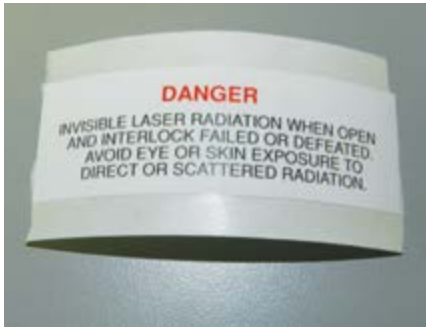
Interlock warning posted by each cover interlock internal to the machine
