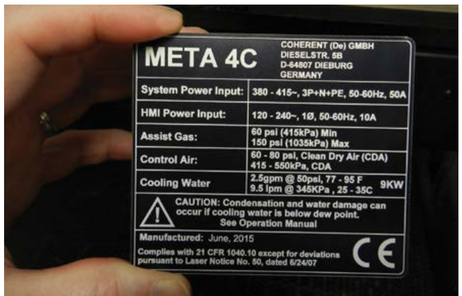
Electrical label on the exterior of the laser machine made of 3mm anodised aluminium
