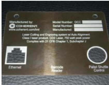
Connector port assembly cut with precise locations holes cut by a laser
