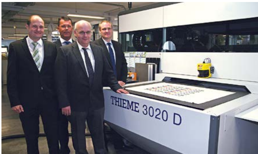
The digital printing unit can be variably equipped with printing heads and offers a resolution of up to 1600 x 2160 dpi.
