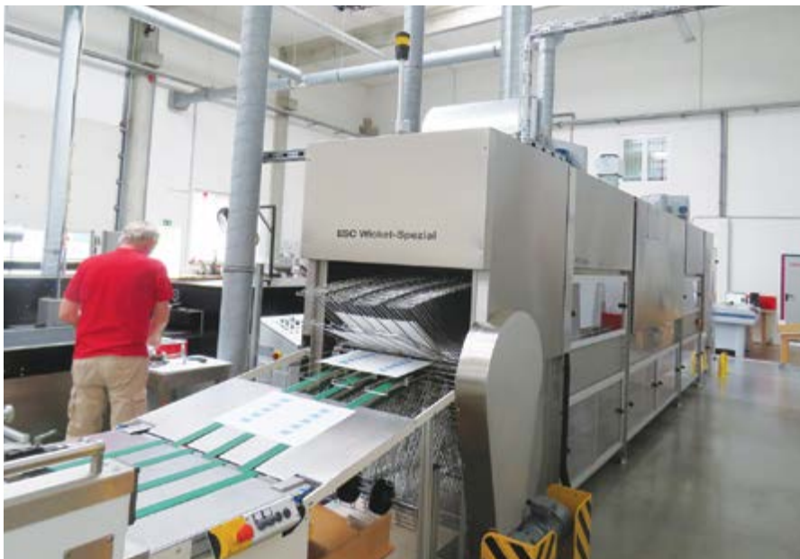
The new ESC-Wicket dryer's special design enables gentle drying of the printed sheets
