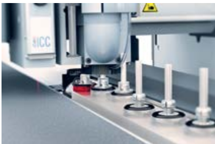
The new collaborative robot does not require a safety cage
