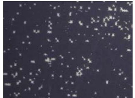
Figure 7: Incomplete print due to ink drying-in problems
