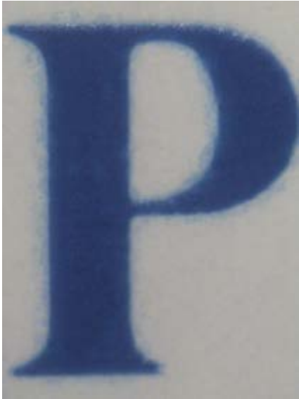
Figure 4: Print showing ink slur on the left side of the image
