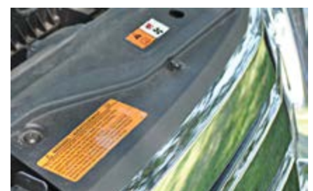
UL labels must demonstrate significant characteristics such as legibility retention, resistance to delamination and adhesion to the surface of the product
