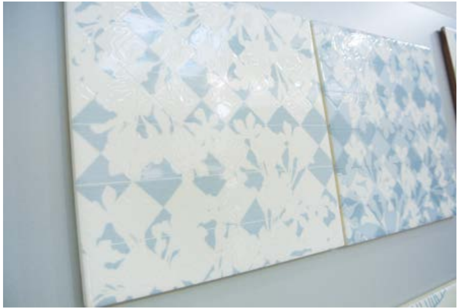
Tile printed glossy white glaze and Smalticeram inks by the TecnoFerrari Vivajet S4 using Xaar 1002 GS40 printheads
