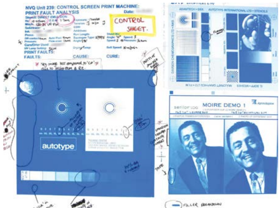
Figure 1: Test print showing faults marked up
