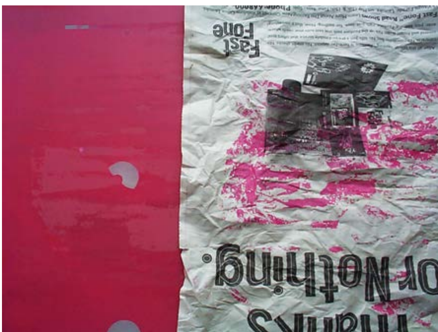
Positives should stop invisible UV energy from reaching the image area
