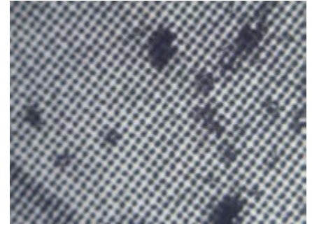
Figure 11: Dust contamination causing 'hickies' in print
