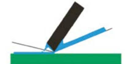
Figure 9: Schematic of squeegee showing how ink teardrops are formed
