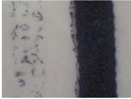
Figure 5: Print showing ink slur and squeegee judder
