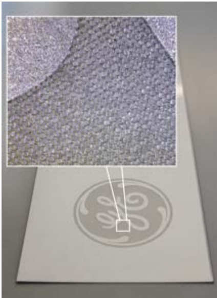
Well-formed round dots (raster) in bold logo, shown under a microscope
