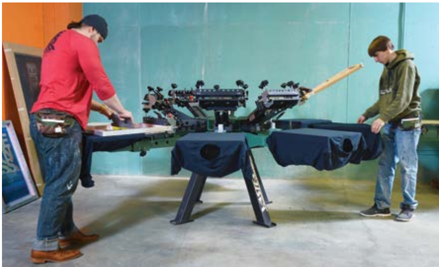
The V2000HD manual press enables all-heads-down printing with two people working on different jobs
