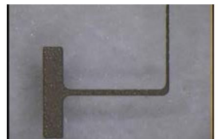
Photo H: 50µm line & space
