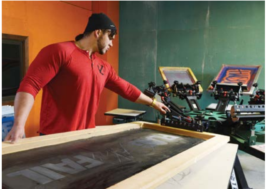
The Vastex manual press accommodates oversize pallets for jobs such as banners
