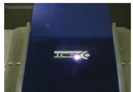
Etching the Inkups Now logo using the Cobalt 1000 YAG laser
