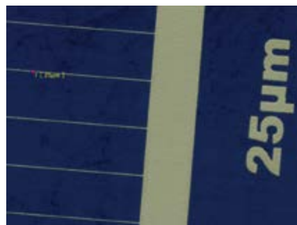
Figure 2: Azocol 170 FL, 25 µm line printed on multi-crystalline silicon wafers – imaged with a light microscope (top) and scanning electron microscope
