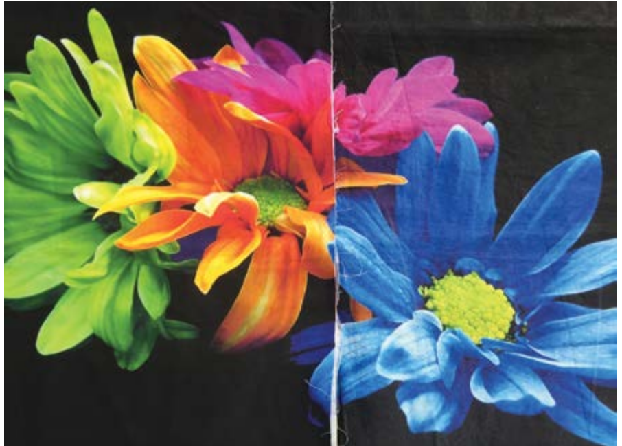
An unwashed pigment pre-treat and a washed at 40 degrees C pigment pre-treat
