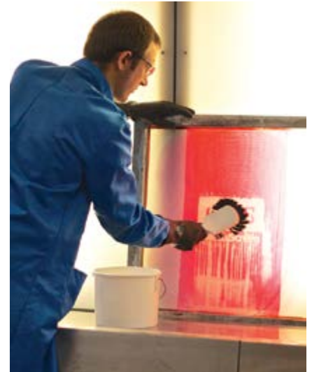
Stencil removers do not contribute to COD of waste water although dissolved emulsions do
