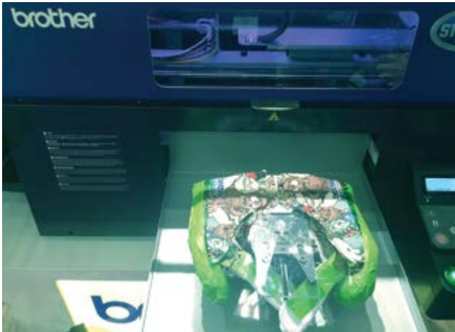
A printed shoe on a speciality shoe platen at FESPA 2015. (Image courtesy Brother Internationale Industriemaschinen GmbH).
