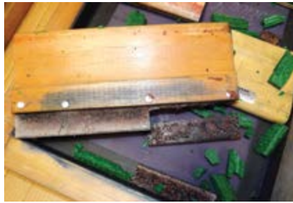
Old squeegees found with some old mesh frames. The dark red and green squeegee blades had become brittle and had broken apart.
