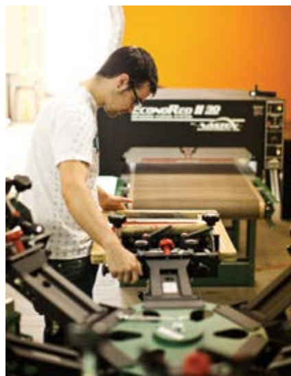
Owner Shannon Thomas makes fine print-head adjustments on his one-colour, one-station press
