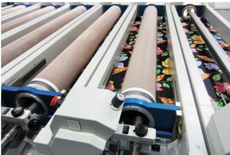
A rotary printing machine with several rotary screen-printing stations arrayed behind each other
