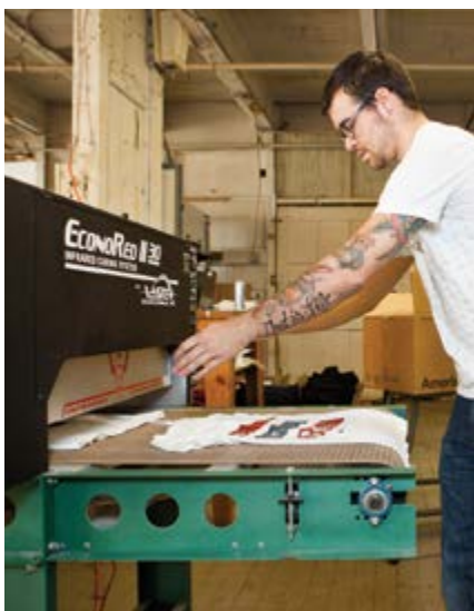
The 76cm infrared conveyor drier allows Four Ambition to tackle oversize printing at faster production rates
