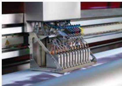
Familiar parts of machines, such as print-heads, should be configured specifically for textile production
