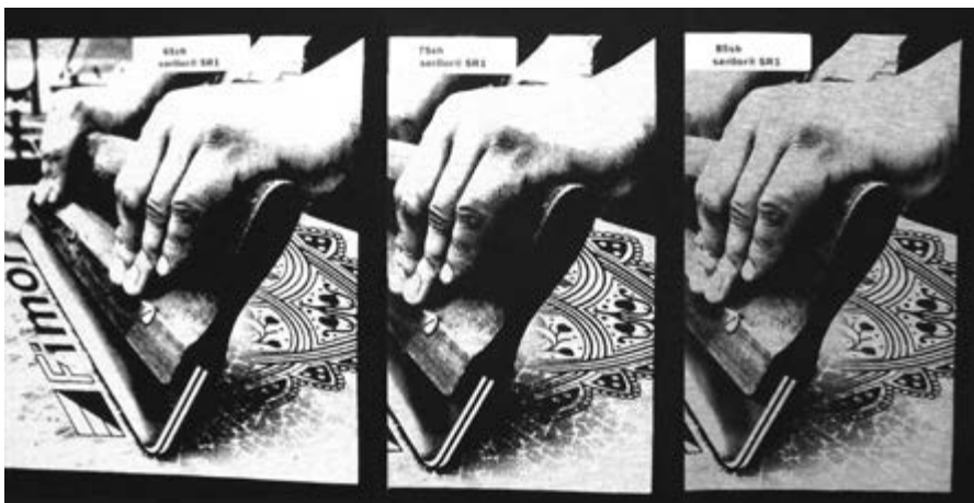
Actual print samples showing how different squeegee hardness affects ink deposit, all else being equal
