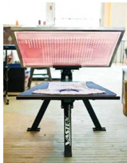
This 46 x 61cm flash drier with adjustable heat control cures oversize prints producing a higher quality finished product
