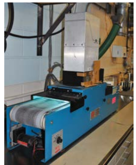
UV light is used to instantly cures adhesives, inks and coatings – traditional heat or air drying methods can take much longer.
