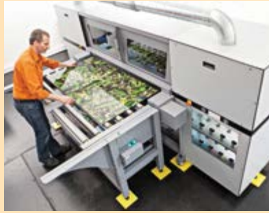
Printing glass treated with the Iris Glass Primer
