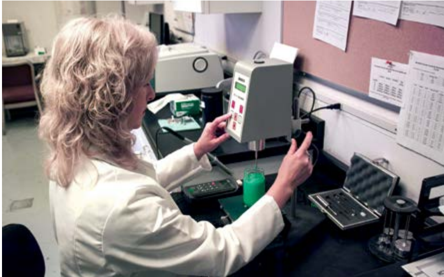
A Chroma Labs chemist reads viscosity measurements of UV-LED emulsion
