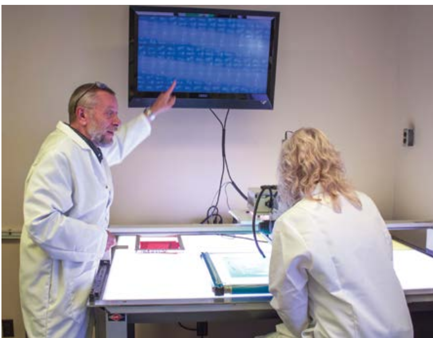
High magnification stencil inspection with video display
