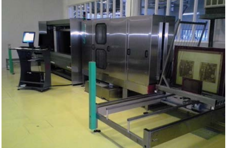
The STM-TEX Pro-10 CTS direct exposing in-line unit produces screens fully automatically
