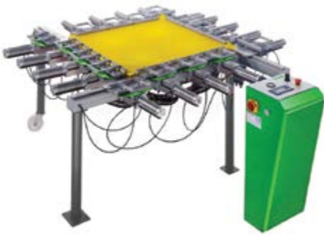
The G-Stretch 215A automatic stretching machine produces standardised screens
