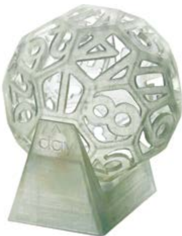
This sample was produced with the Roland ARM-10 3D printer and shows how hollow and complex shapes can be created
