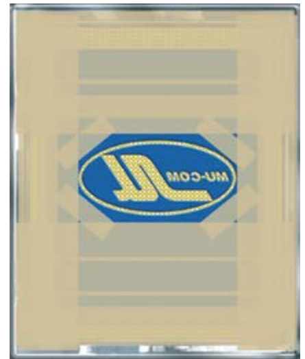
An example of a screen with too much tape
