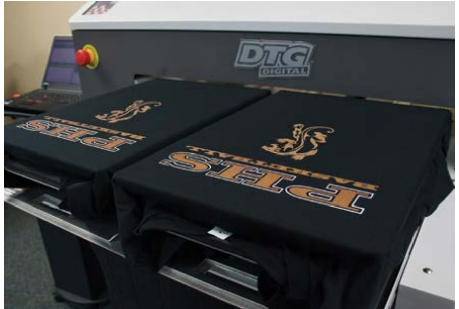
Digitally garment printing a short-run part of a screen-printed order
