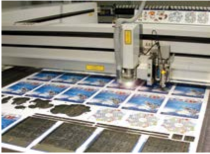
Laser cutting of printed textile from Georg + Otto Friedrich with the help of the Camera Recognition System and the Conveyor System
