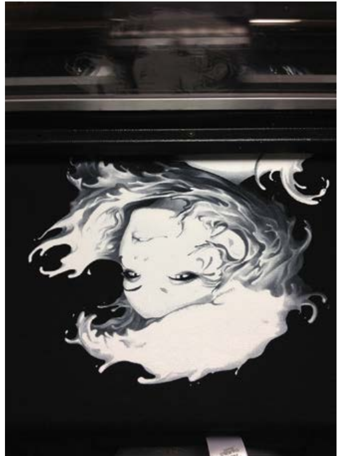
Using water-based digital textile white ink can produce prints that challenge screen-printing
