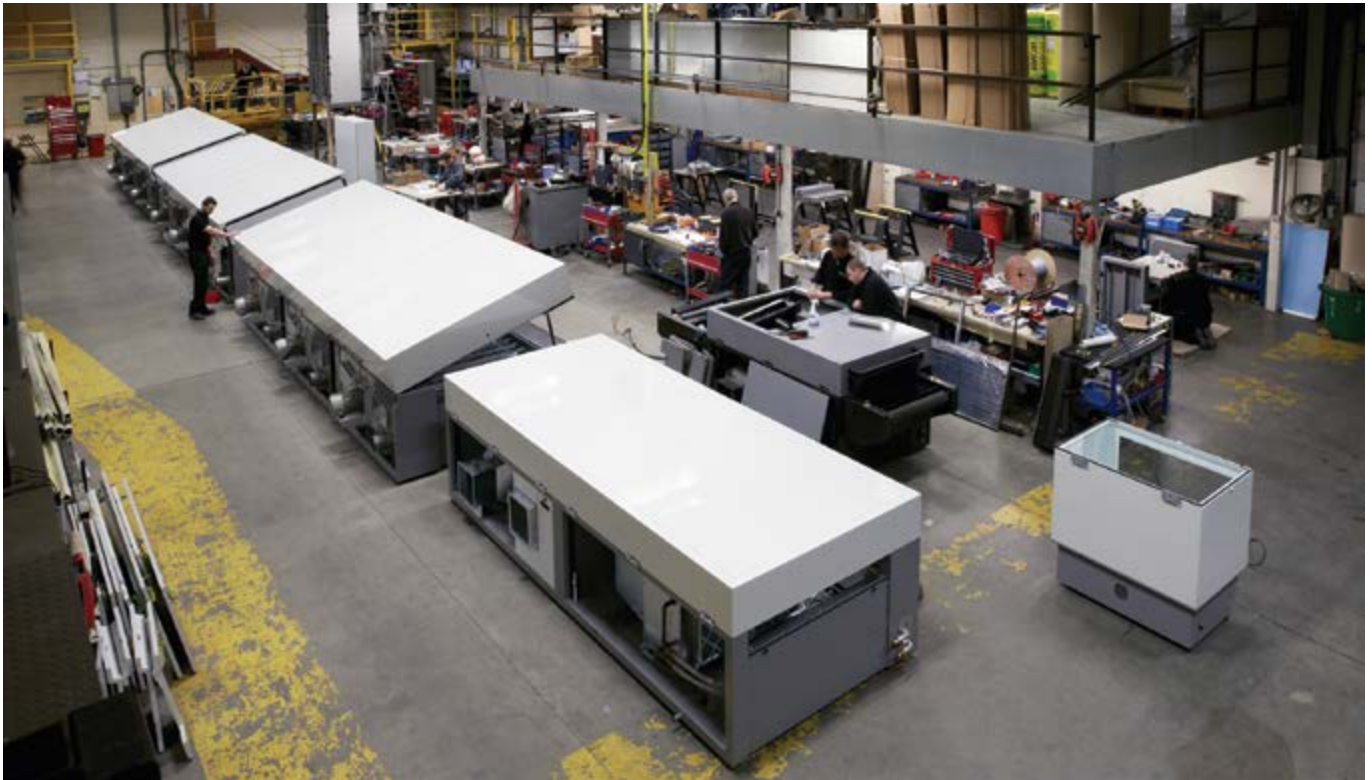
The assembly of Natgraph's longest ever, 30m dryer at 30m
