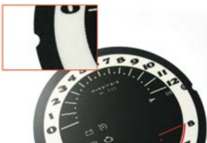
Laser cutting of printed foil including the detailed cut edge
