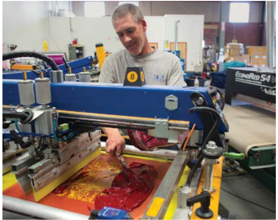
For higher volume runs, co-owner Brian Haines operates an eight-colour, ten-station automatic press
