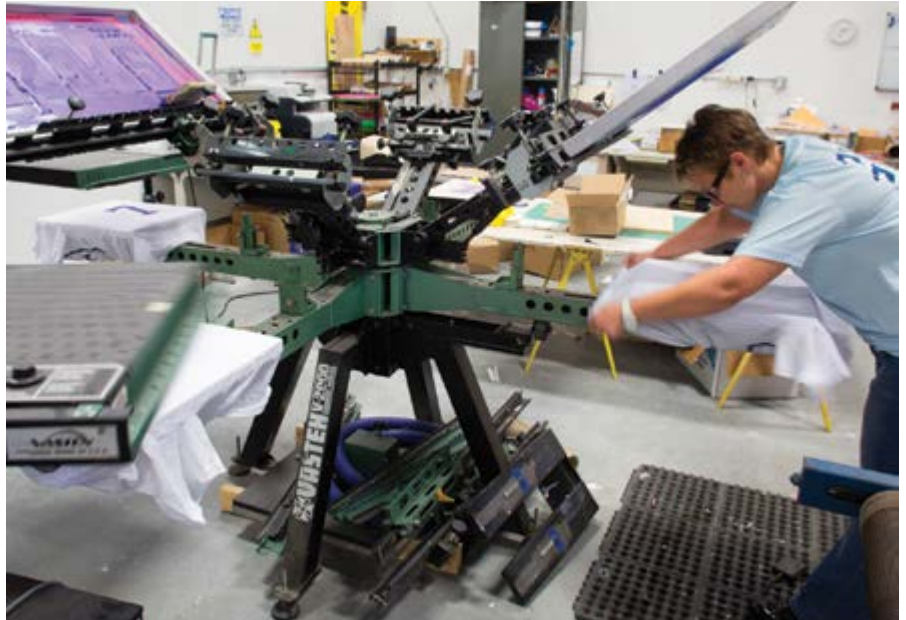
Fitting a shirt to the V-2000 four-station, four-colour manual press. Left: an infra-red flash cure unit dries items between stations. Back left: the DiGiT athletic numbering system
