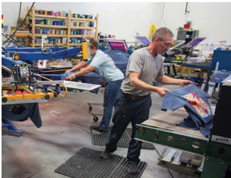
Keeping pace with the automatic press, MiddletownInk dries garments with an EconoRed II infra-red dryer that has a 137cm wide belt
