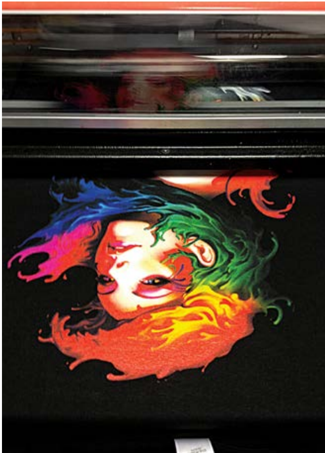
A bright white under-base allows for vibrant colours
