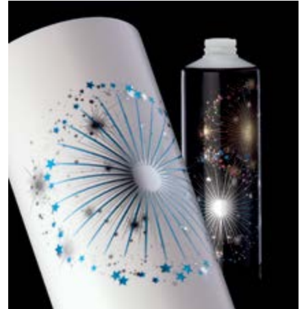
High resolution images can be in-line foiled onto extruded tubes
