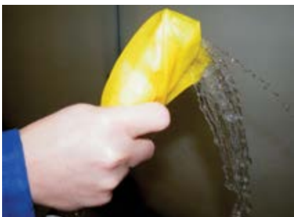
Using a mesh as a filter cloth to check for waterborne contamination
