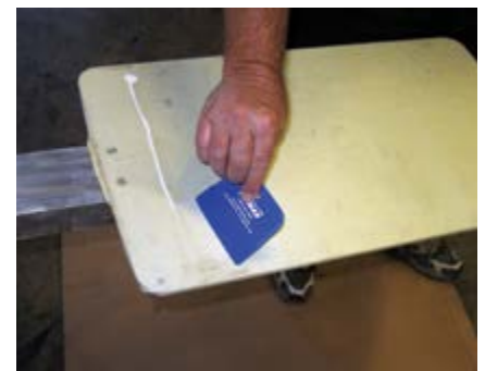
Spreading table adhesive
