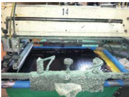
A soft furry coating can infiltrate every nook and cranny of the press
