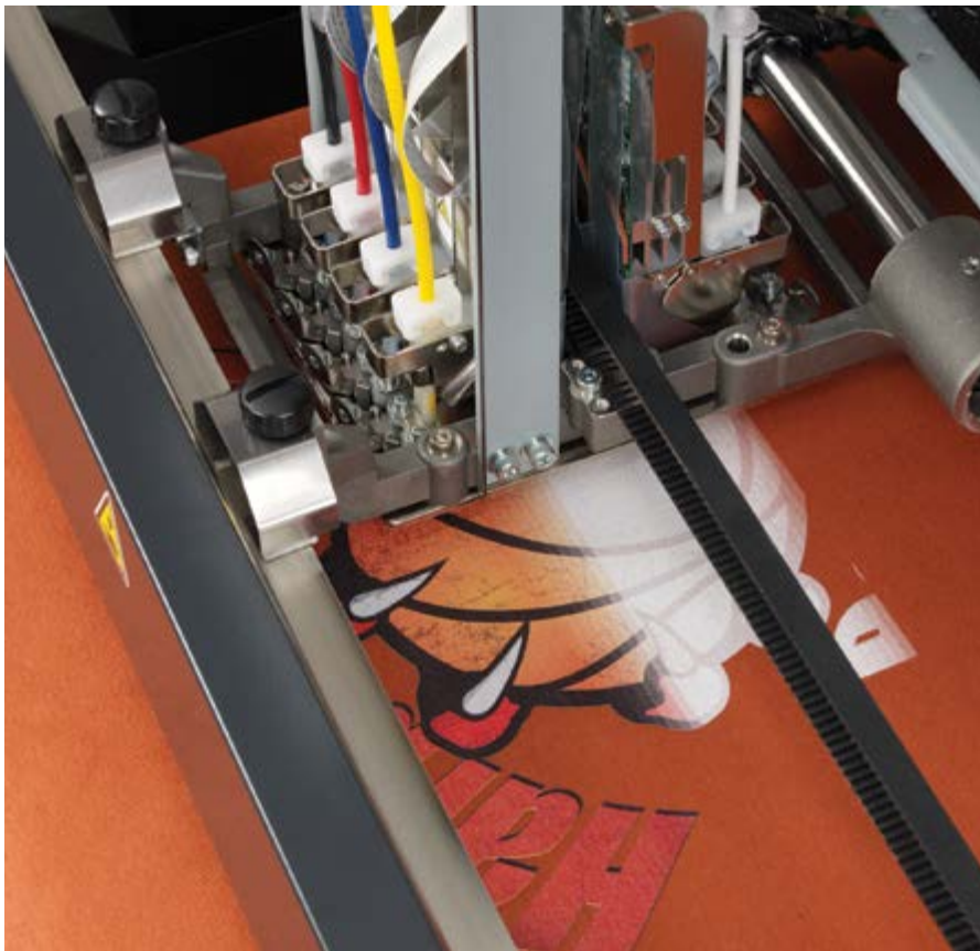
Printing CMYK and white direct with the Brother GT-3 Series
