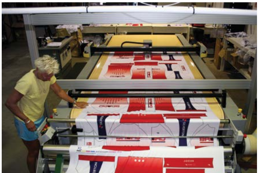
The Gerbercutter and ContourVision scanning system in action
