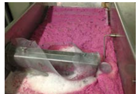
High sludge formation in an inline sloping filter system
