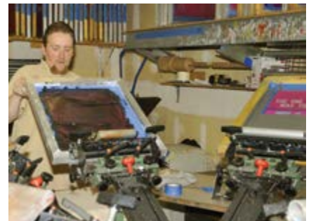
The print head allows tool-free micro-registration, head levelling and off-contact
