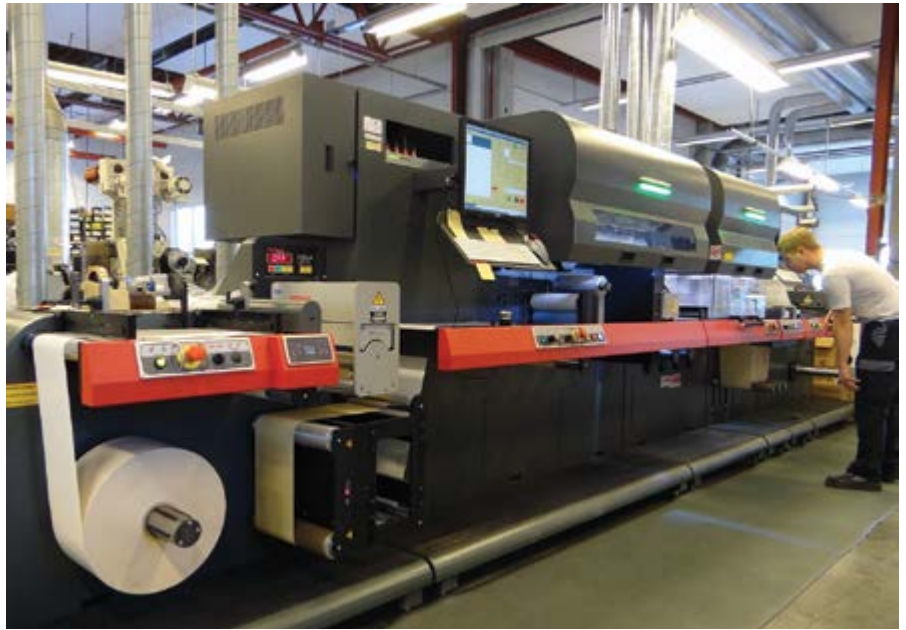
The Jetrion 4900 has a compact foot-print of just seven metres, including unwind and corona treater
