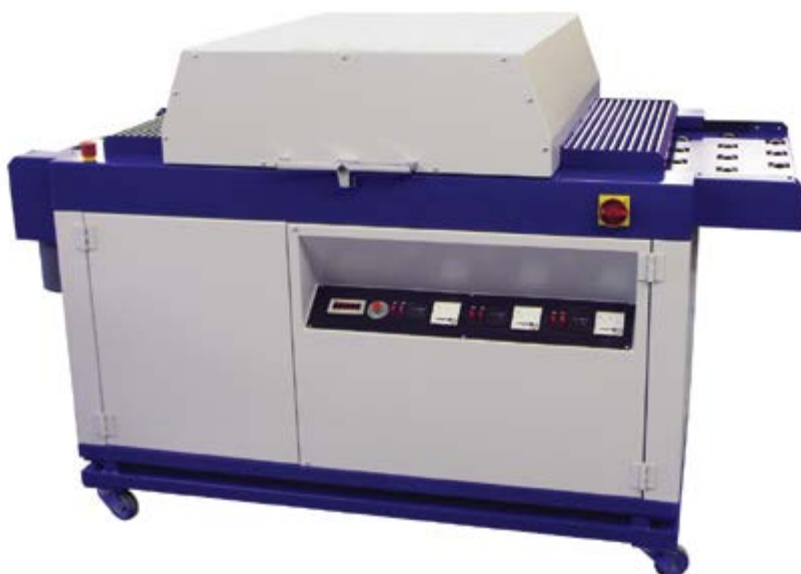
The AKTIPRINT G is suitable for the UV curing of lacquer or for UV sensitive ink and colours
