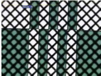
Line widths as fine as 20\mu\text{m} are consistently possible with Azocol Z 170 photoemulsion
