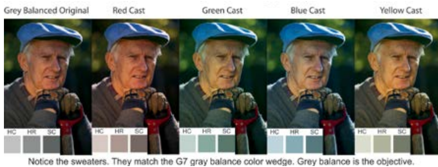
Figure 2: Correct grey balance image and four images with a colour cast
