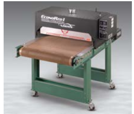
Two EconoRed I models with 167.6 cm belt length are recommended for small- to medium-size shops: an EconoRed I 30 with a 76.2cm wide belt and new 4300 Watt heater (shown) capable of curing 190+ pieces/hour/chamber and the EconoRed I 54 with a 137cm wide belt capable of curing 380+ pieces/hour/chamber
