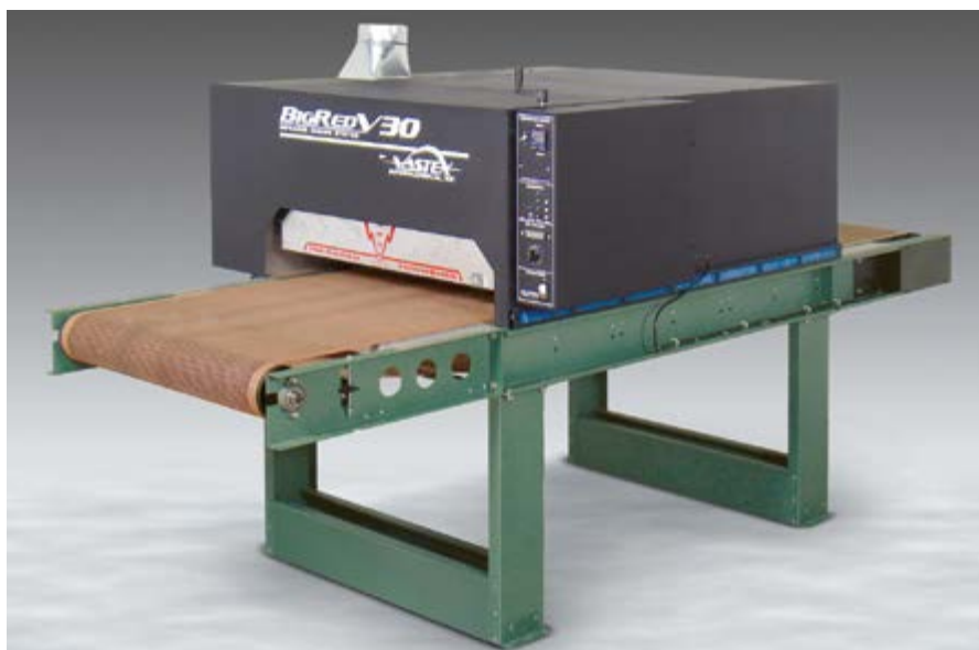
Figure 2: BigRed V30 models (76.2cm belt width) can dry 475+ plastisol-printed pieces, 200+ water-based-printed pieces, and 56 digital-white-printed pieces per hour/chamber. BigRed V54 models (137.2cm belt width) can dry 950+ plastisol-printed pieces, 400+ water-based-printed pieces, and 112 digital-white-printed pieces/hour/chamber.
