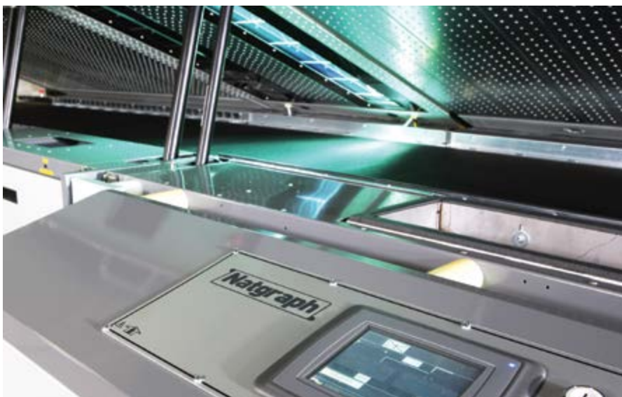
A Natgraph UV system with PLC control
