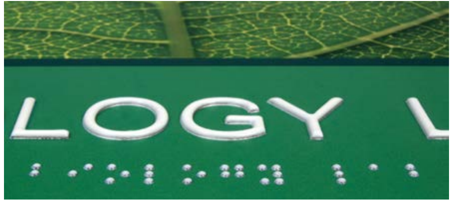
Raised objects printed on top of a flat UV LED print
