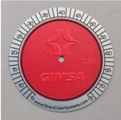
A raised object with a flat UV LED print over the top provides an embossed look
