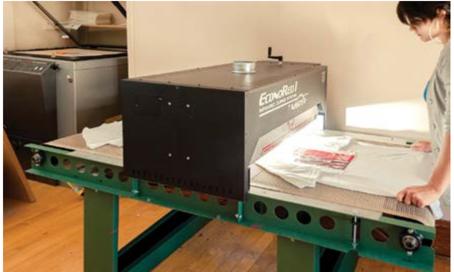
Figure 1: this Vastex BigRed I infra-red conveyor dryer is used to cure inks on shirts, hats, signs, tote bags, bumper stickers, vinyl labels, binders, hockey pucks, metal parts and other screen printed items at high rates
