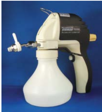
This spot cleaning gun has an integrated air dryer
