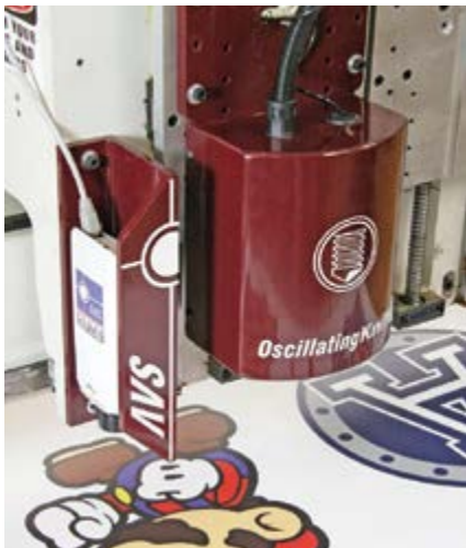
Precision alignment for cutting out pre-printed materials with XYZ's AVS camera registration system
