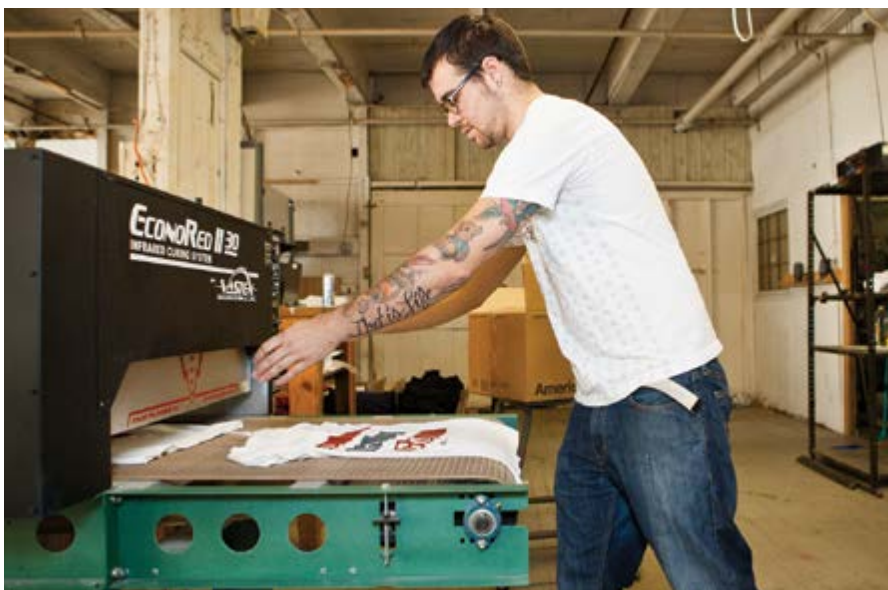
This 76 cm EconoRed II infra-red conveyor is utilised for drying of plastisols, water-based and discharge inks, and heat transfers
