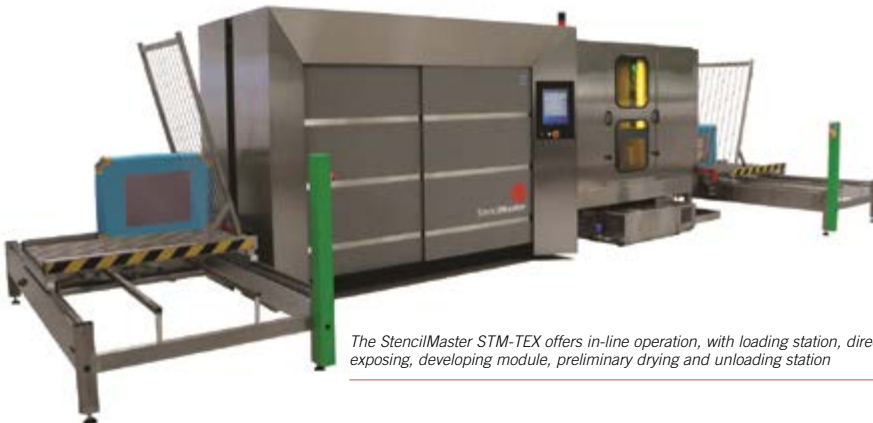
Computer-to-screen (CIS) with in-line automation v conventional screen-making
