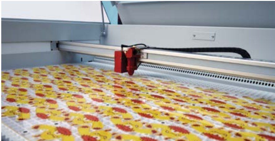
Above and right: the Trotec Speedy 400 with Esko Artwork's i-cut Vision registration system
