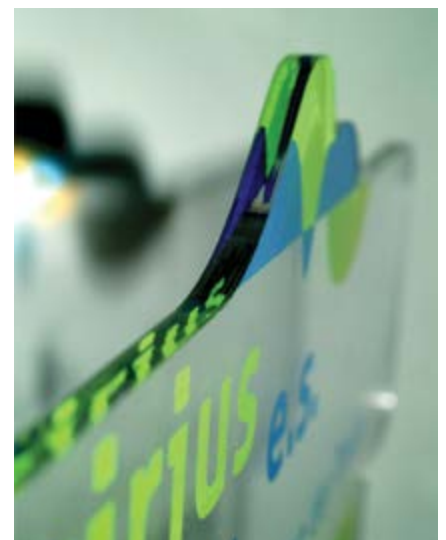
Flame polished laser-cut edges produced without polishing
