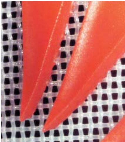
3D effects are achieved with a high stencil profile of greater than 200 microns and the appropriate mesh
