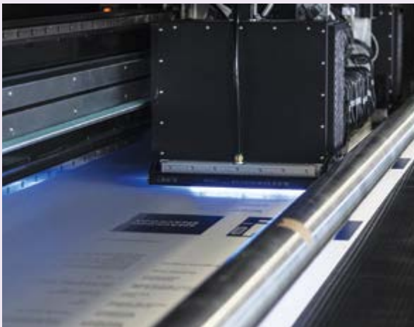
EFI's VUTEK GS3250LX is an example of a successful wide-format printer that incorporates LED curing
