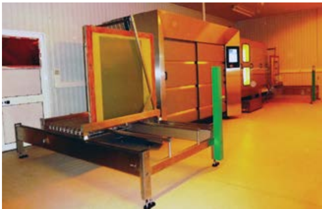
Integration of the G-Wash 175 XS and STM-TEX as a complete CtS and developing line
