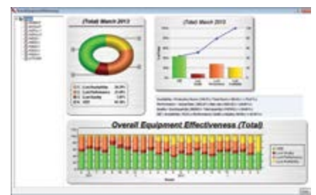
The key performance indicator screen, highlighting overall equipment effectiveness
