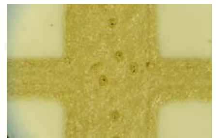
Figure 7: Commercial screen-print silver ink at >10 microns thickness made up of micron-scale flakes after application of standard-structure photonic curing pulse. Note the occurrence of crater-like surface structures
