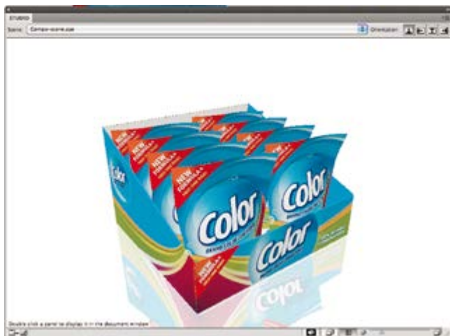
ArtiosCAD lets users fill a carton, case or tray with the product being packed
