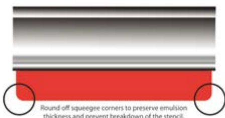
Figure 6: Rounded off squeegee corners
