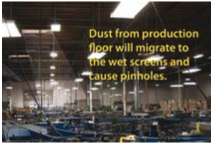
Figure 5: Shop dust causes pinholes
