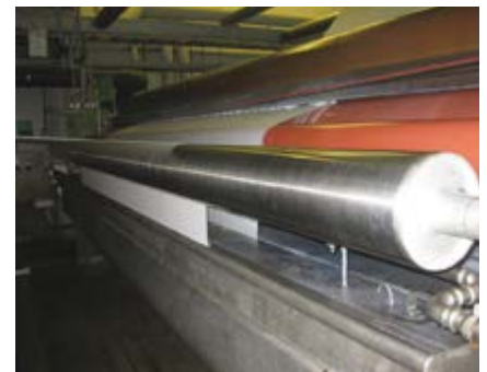
Coating machine applying the ink-receptive top-coat.
