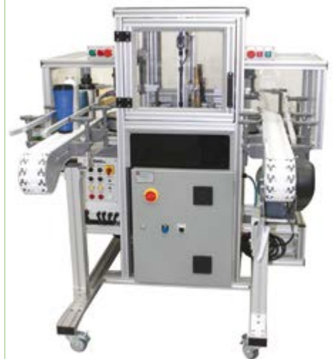
Figure 5: a custom built pre-treatment conveyor flamer
