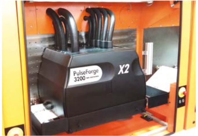
The PulseForge 3200-X2 integrated into a roll-to-roll processing tool
