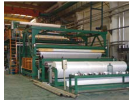
Laminating machine bonding PVC facestock to scrim with roller pressure and heat
