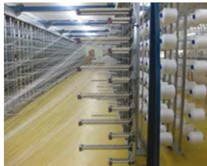
Polyester yarns being spun together to create the knitted or woven scrim [scrim.tif]
