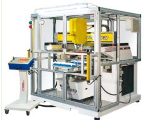
Figure 3: a servo-driven pad printer with PC controller
