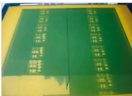
The effect of insufficient mesh preparation
