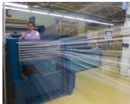
Woven scrim construction. PES yarns feeding into weaving loom
