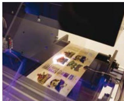
Laser cutting stations in-line with digital printing equipment are allowing label manufacturers to introduce 'lean manufacturing' practices throughout their plant.
