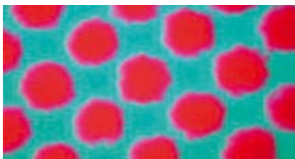
Figure 1: An example of a good dot, with no leaks, bleeding or thread interference
