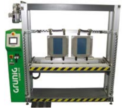
The G-Coat 415 automatic coating machine is designed for various screen sizes.
