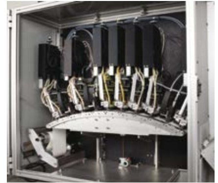
Technology breakthroughs utilising seven XAAR print stations including a pre-coating station, CMYK White print stations, UV varnish station along with UV pinning lamps and a final UV cure are being introduced onto the marketplace.
