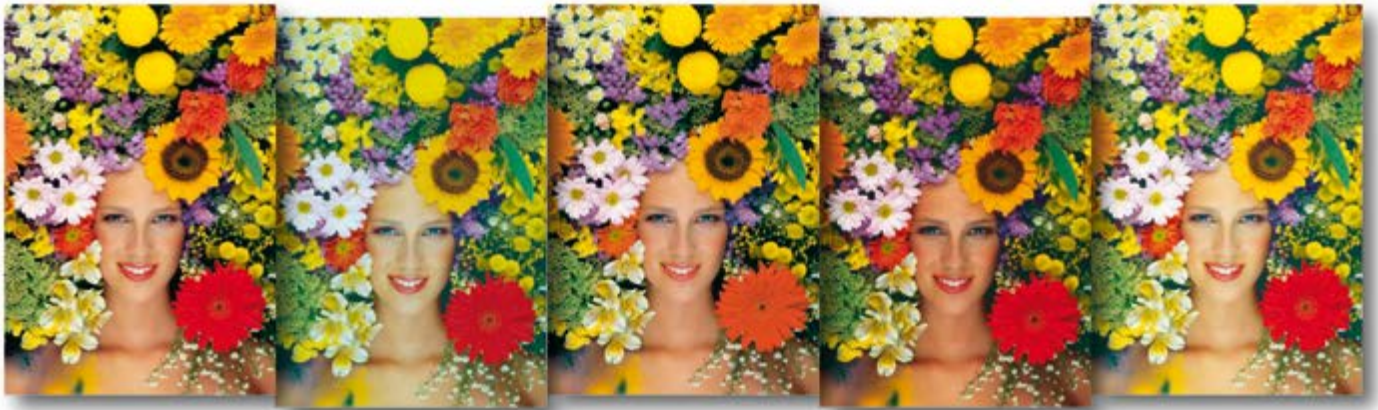
Colour casts caused by incorrect separations
