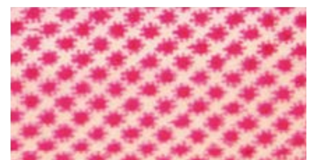
Figure 6: An example of ink leaking all the way around the dot
