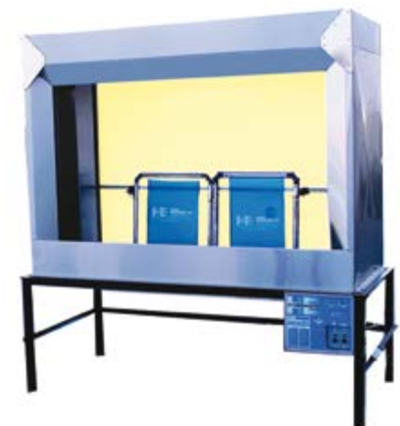
A dedicated degreasing and development sink reduces screen contamination
