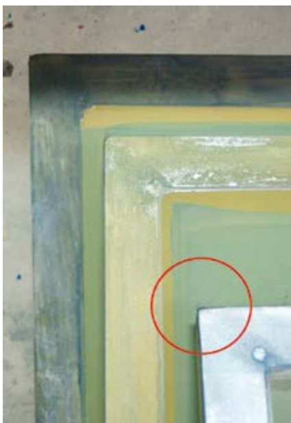
Frame corners can damage fine meshes
