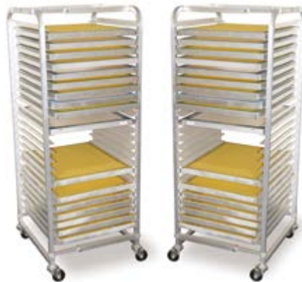
Screen racks serve an important function by preserving mesh
