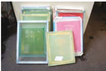
It's important to avoid resting frame corners against the mesh
