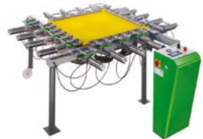
Grünig-Interscreen’s G-Stretch 215A stretching machine
