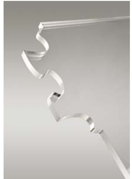
The smoothness of routed acrylic reveals vibrations and can be taken as an indication of the system's robustness
