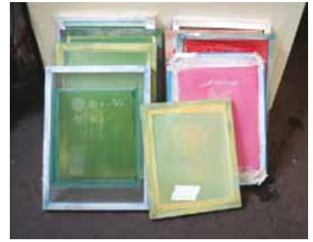
Poor screen handling procedures
