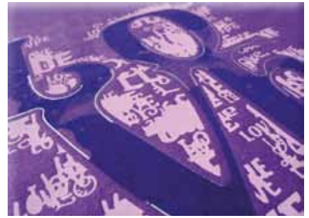
A transfer paper base with torn off flock outlined with reflective material
