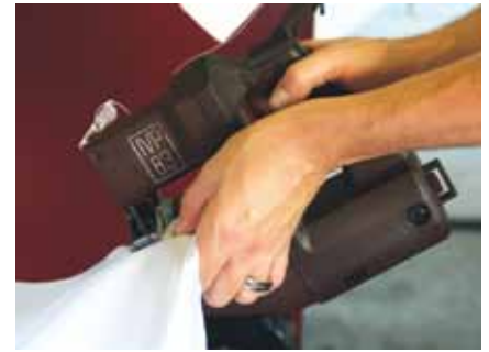
A hand-held sewing machine makes it quick and easy to join rolls
