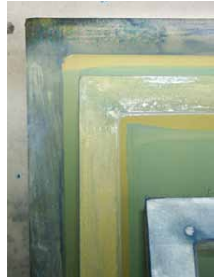
Resting screen corners against mesh will damage screens
