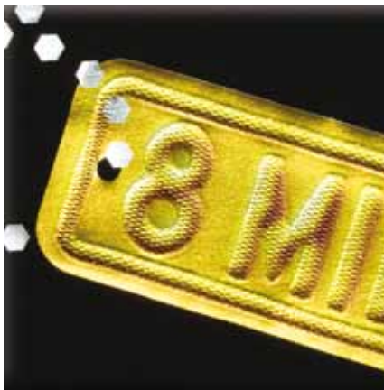
This metallic layer is raised due to a puff layer underneath it, creating a 3D effect
