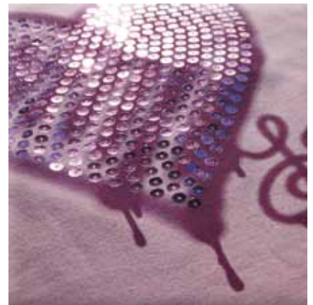
Combining a direct-to-garment outline and a holographic heat transfer material to mimic a rhinestone effect
