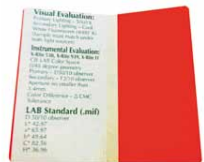
This is a photograph of a typical color card. On the left is the specification of what the color values should be. The right side is a sample of the color to be used visually to control a clients brand color. The problem is... the color on the right does not match the numbers on the left.
