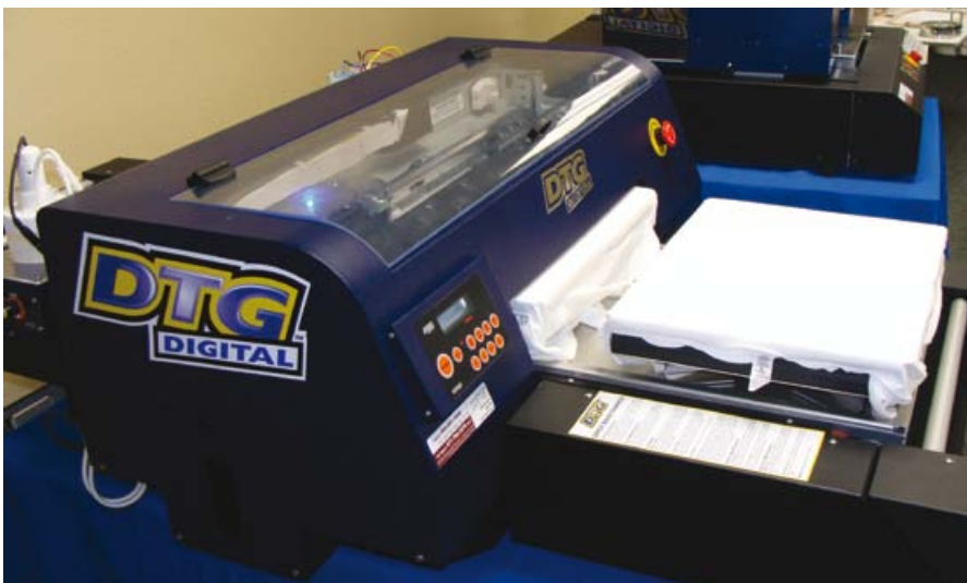
A direct-to-garment printer outputting two white garments
