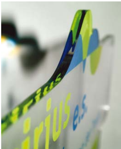
Flame polished laser cut edges produced without polishing
