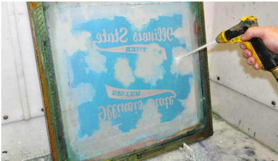
Example of what happens when a hot solvent has been used for cleaning the ink from the screen
