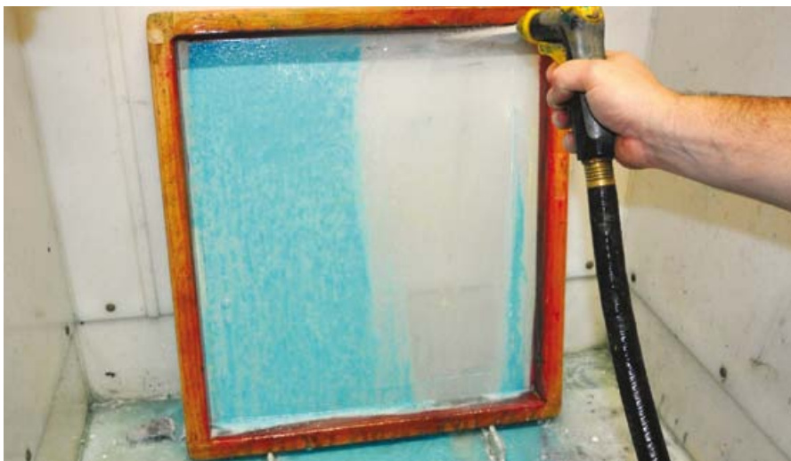
When proper ink cleaners have been used and the correct emulsion remover is used to reclaim, the emulsion will clean easily
