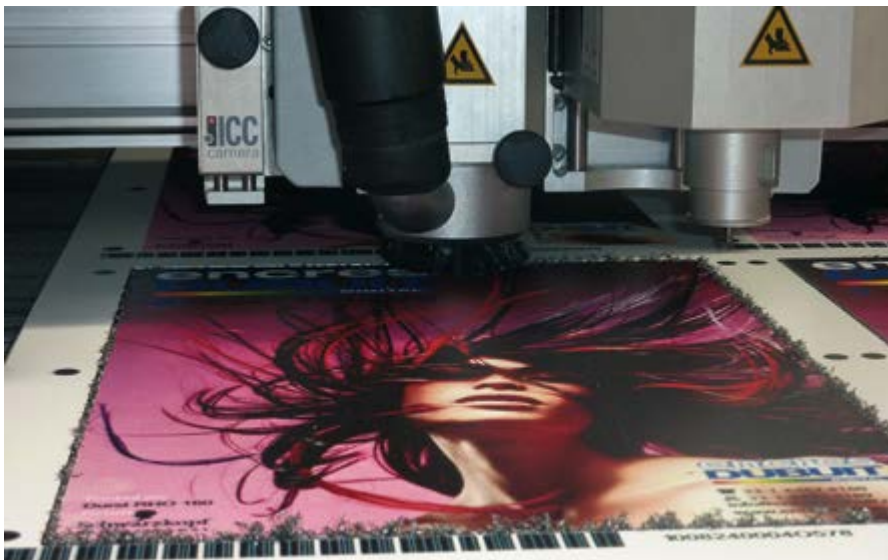
This ink is claimed to exhibit great flexibility and good adhesion on DiBond and other rigid substrates, and this also facilitates die-cutting
