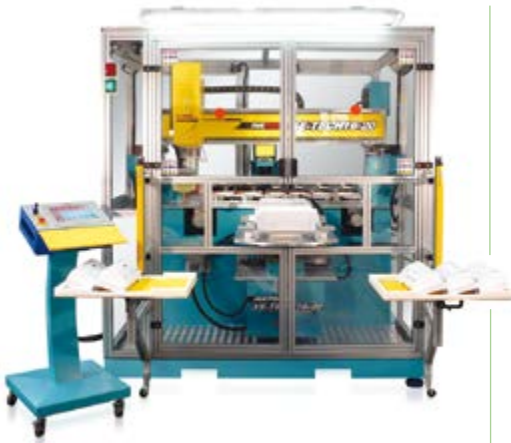
Figure 4: One pad printing machine with multiple pads and colours can print a large format part such as this appliance panel in one machine cycle.
