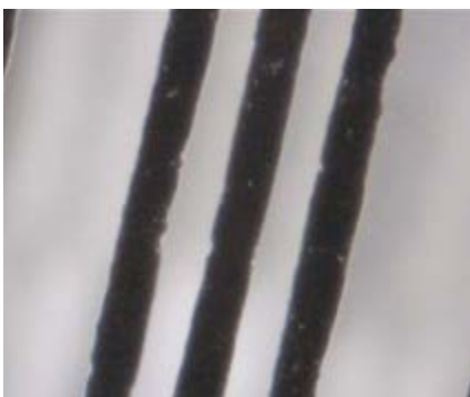
Print result with an EOM of 7 microns and an Rz value of 5 microns. Seen at 140 times magnification
