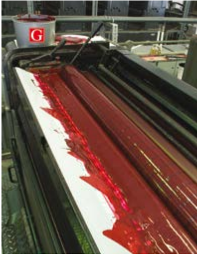
Gans sublimation offset inks on a Heidelberg offset press
