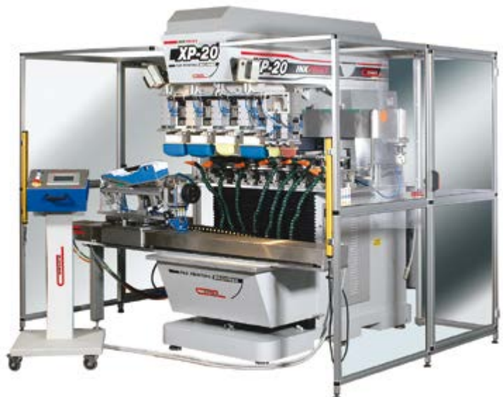
Figure 3: Using a pad printing machine is a quick and effective method for direct printing on large format, irregular and three-dimensional parts.
