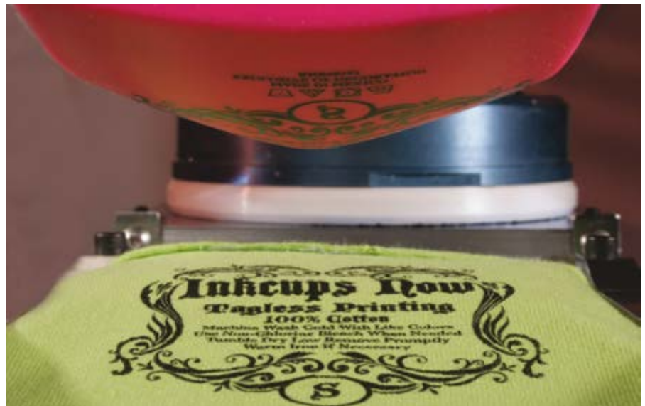
An example of a neck tag pad printed with the B-100
