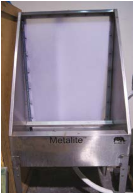
Dedicate one wash-out booth for reclaiming emulsion and washing water-base screens, and another for degreasing and screen development
