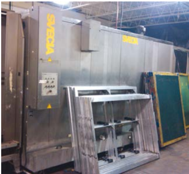
Svecia in-line screen reclaiming machine (Up North Trading Company in Lakeville, MN USA) using 'One Step' technology
