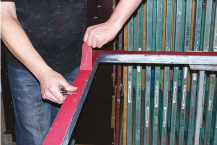
Old, well enduring, coherent adhesive layers can be left on the frame for new stretching
