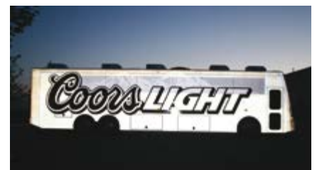
Retro-reflective window graphics are also visible at night when light strikes them Photo courtesy of Graphic Impressions, Vancouver, BC
