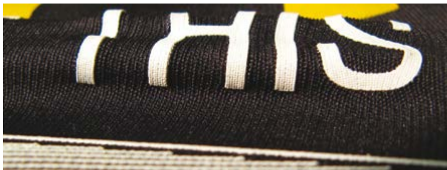
A print on performance fabric with elastic fibres using a stretch additive
