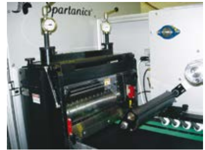
The Spartanics Finecut-Plus-Rotary combination laser die cutting and rotary die cutting system
