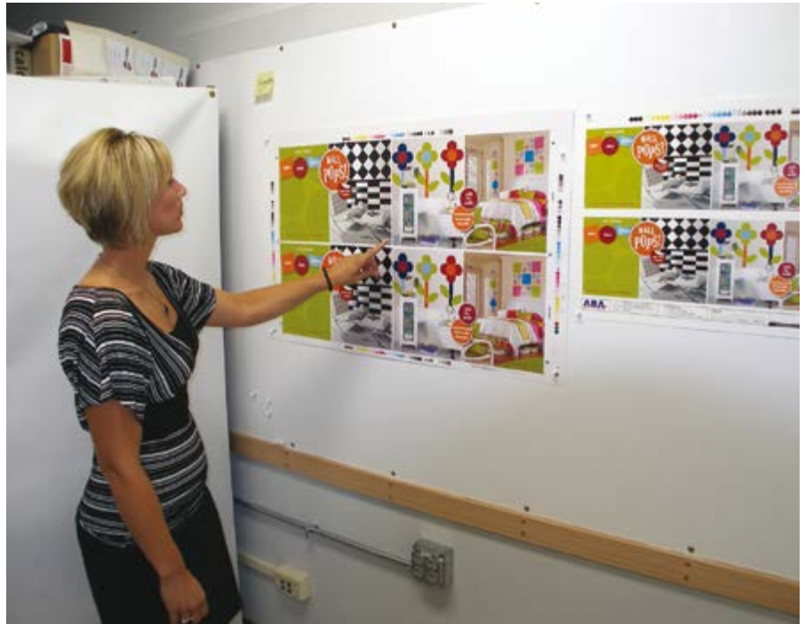
When proof and print are composed of different elements, the best result is one of a 'common appearance' as targeted in G7 methodology
