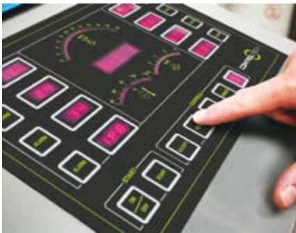
The flexibility of the ink means that operating panels can be produced successfully
