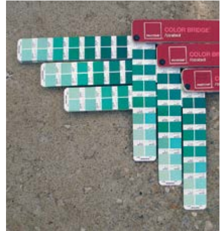
These Pantone Bridge books are all the same type and age of book. But, due to variations in the manufacturing process, there will be an acceptable deviation in the colours expressed in a Delta E tolerance
