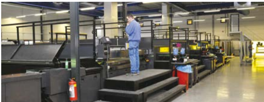
The screen-printing line, four colours at the time – prettier, faster and cheaper
