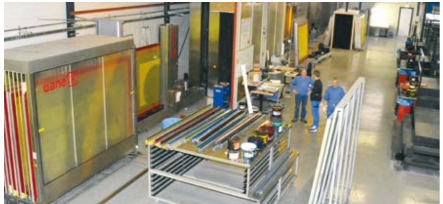
The frames slide automatically into the line to come out clean 35m further after having been coated, exposed and dried
