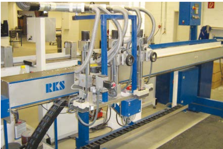
The SM2800 AL multi head squeegee grinding machine
