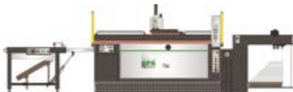
The SPS Vitessa SL2 with, on the left, the SPS RSS 2 reject sheet selector
