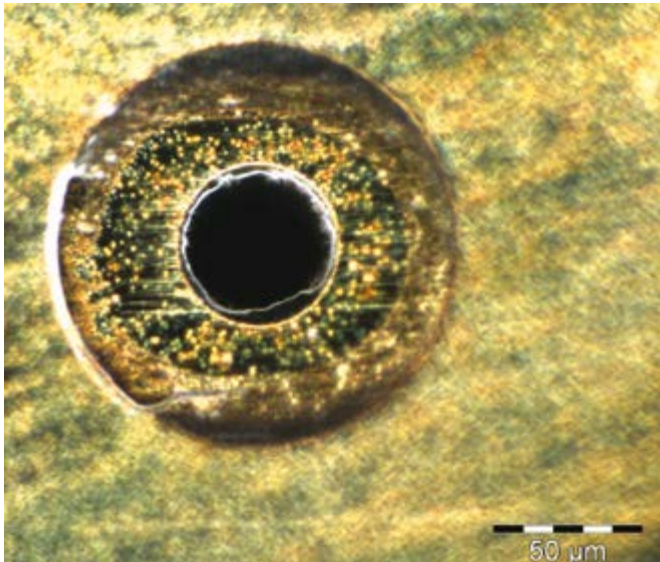
Figure 2: A print nozzle under an optical microscope
