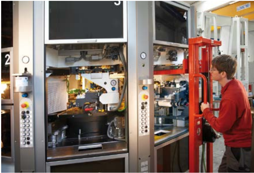
Printing units can be exchanged easily using a specially adapted hand winch cart
