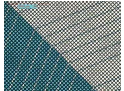
Azocol Z 175 photoemulsion can achieve a resolution from 20-50 µm, both in positive and negative
