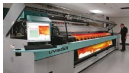
The Uvistar series of UV inkjet roll to roll printers has been developed for PE single skin billboard posters
